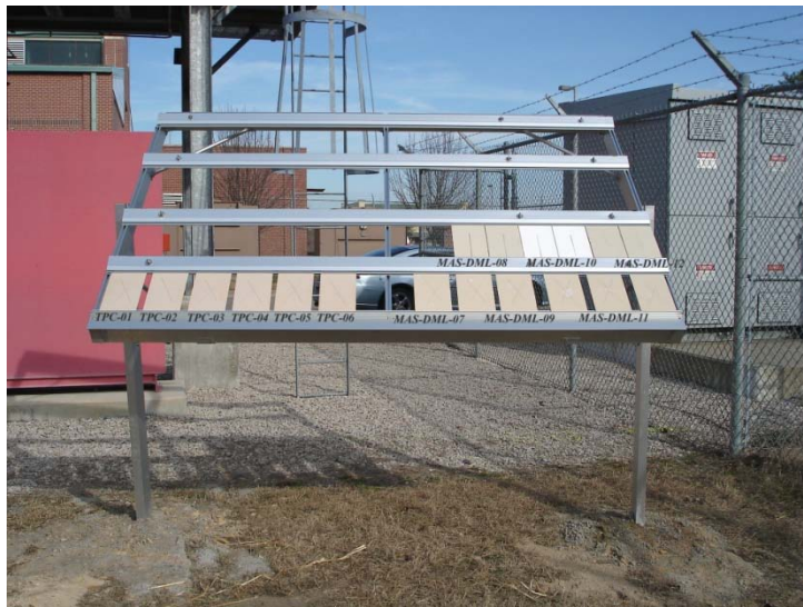
Figure 20. Exposure rack with coupons prepared with the coating systems used on tank #2.
