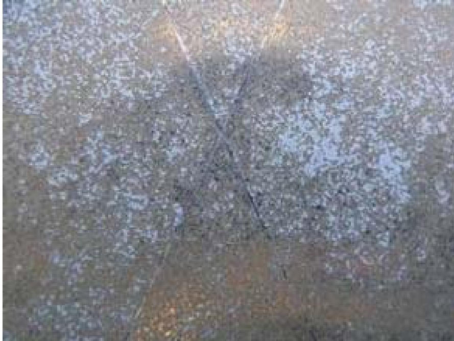
Figure 6: XP-406 on AA 2024 without a topcoat after 8 months exposure at KSC.
