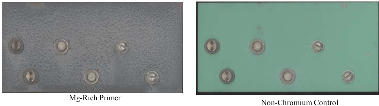
Figure 15: XP-417 and non-chromate control galvanic test panels without a topcoat after 4 months outdoor exposure at KSC.
