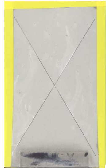
MIL-DTL-81706 Type II – Trivalent Chromium (Alodine T5900)
