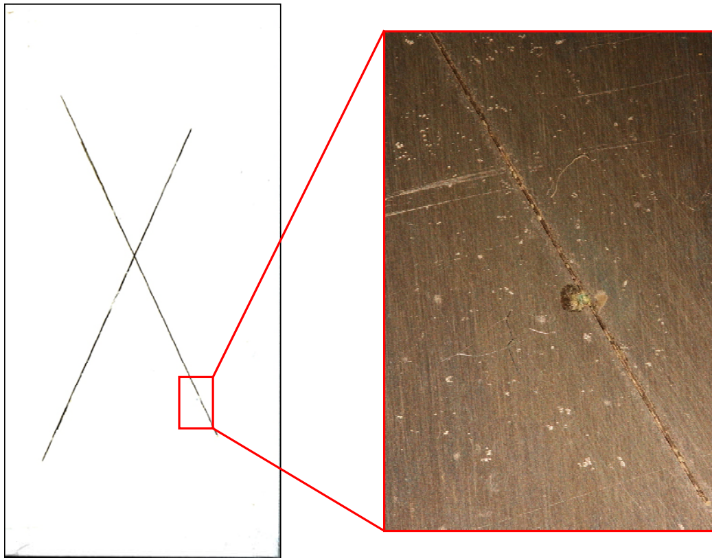
Figure 16: Aerodur 2100 MgRP with a topcoat on AA 2024 after 2000 hrs. ASTM B 117 neutral salt fog, along with a close-up view of panel after coating removal.
