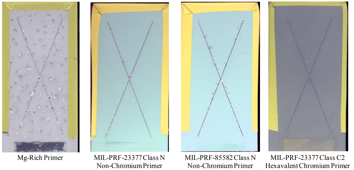
Figure 9: The XP-417 and other control coatings on AA 7075-T6 after 1500 hrs. ASTM G 85.
