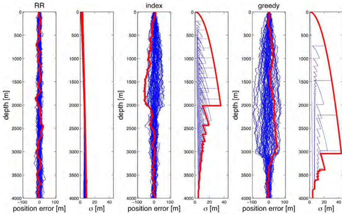
Figure 5-14: Performance of index, RR and greedy algorithms with the extreme weighting function  $T = z^{20}$ . Vehicles are spaced 200 seconds apart. The blue lines are the trajectory of all 50 vehicles as a function of depth. The left plot of the pairs shows horizontal position (simulated), and the right plot shows the tracking uncertainty as predicted analytically by the KF.
