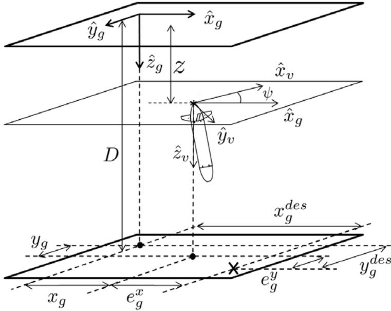
Figure 2-3: 3D coordinate frames used for flight control with surface camera. The global frame  $\hat{x}_g, \hat{y}_g, \hat{z}_g$  is centered at the location of the surface raft. The body-referenced frame  $\hat{x}_v, \hat{y}_v$  and  $\hat{z}_v$  is aligned with  $\hat{z}_g$  but is rotated in the horizontal plane by the vehicle's compass heading,  $\psi$ .
