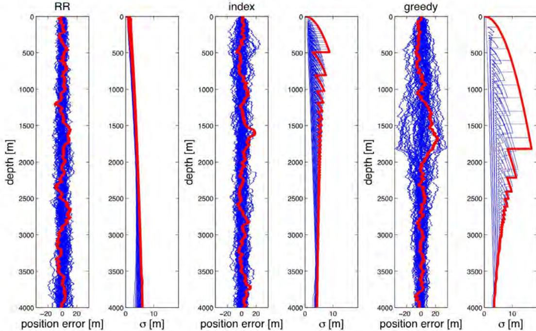
Figure 5-13: Performance of index, RR and greedy algorithms with weighting function  $T = z^4$ . Vehicles are spaced 200 seconds apart. The blue lines are the trajectory of all 50 vehicles as a function of depth. The left plot of the pairs shows horizontal position (simulated), and the right plot shows the tracking uncertainty as predicted analytically by the KF. Jumps in the uncertainty correspond to measurements of that vehicle.
