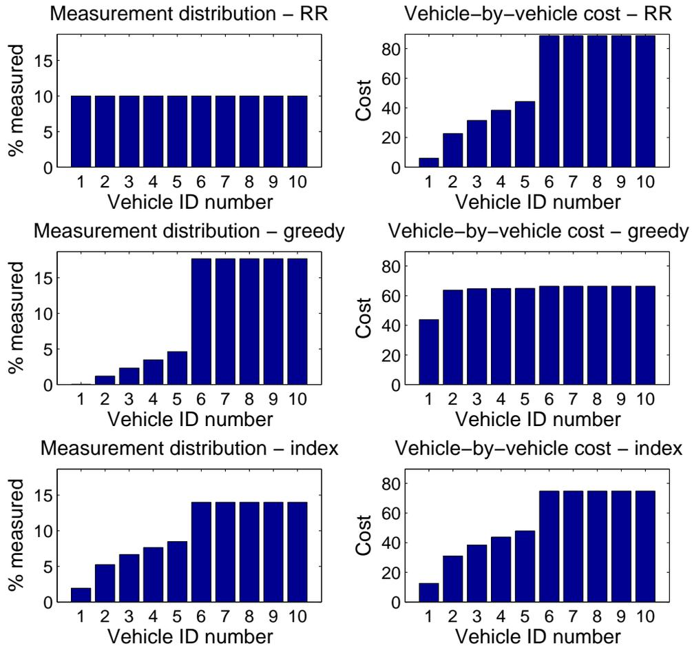
Figure 5-8: Case 3: measurement and cost distributions,  $N = 10$  and  $T_f = 10,000$  sec. The left column shows the measurement distribution—the percentage of total measurements given to each of the 10 vehicles by the scheduling policy. The right column shows the corresponding contribution to the total cost of each vehicle, given the scheduling policy. The rows correspond to the RR, greedy heuristic and RBKF index algorithms.
