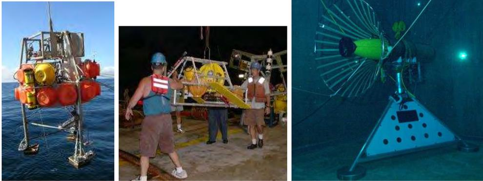
(a) IFM Geomar Lander (b) WHOI Steerable Elevator (c) MBARI AUV Docking vehicle
