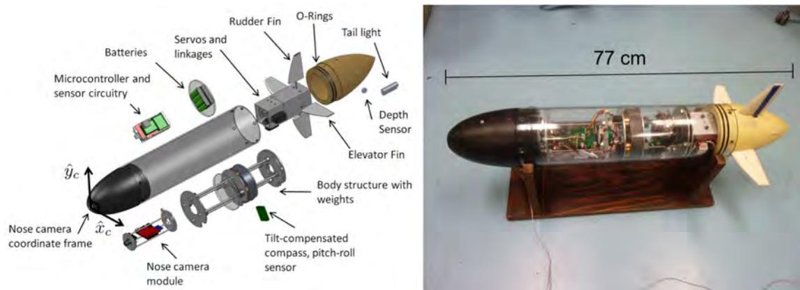
Figure 2-1: An exploded view of the vehicle is on the left, including the onboard camera reference frame  $\hat{x}_c$  and  $\hat{y}_c$ . A photograph of the vehicle with the communication tether attached to the side of the nose is on the right. Note the large lead weight near the center of the vehicle which was located to place the center of mass very slightly below the center of buoyancy, resulting in a marginally stable vehicle that can fly at high angles of attack.
