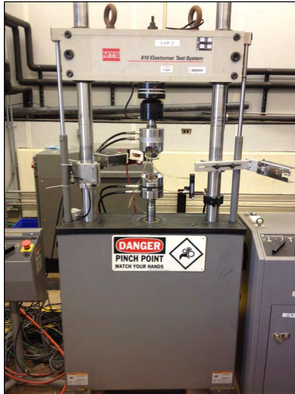
Figure 27. 5 kips MTS machine
