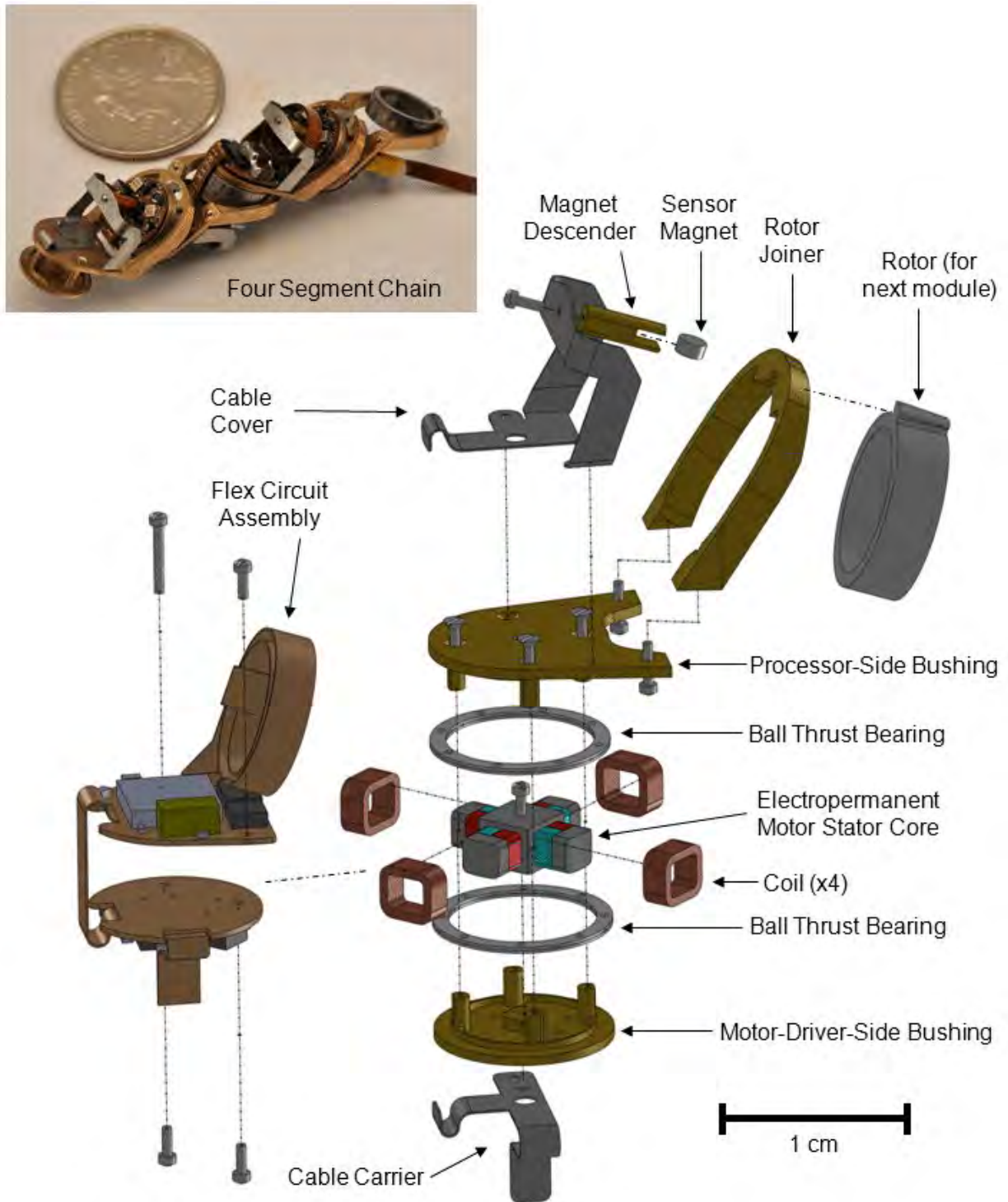
Milli-Motein Module Exploded View. This assembly is repeated for each joint. One segment of the continuous flex circuit is shown in its folded configuration. The stator on this module mates with the rotor on the adjacent module.
