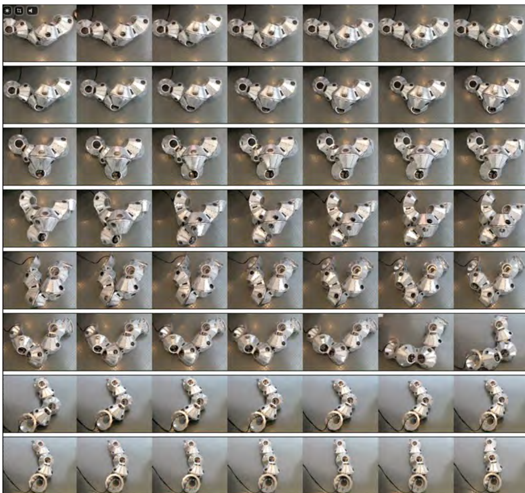
Macrobot fold sequence from a line to an arbitrary shape and back to a line.
