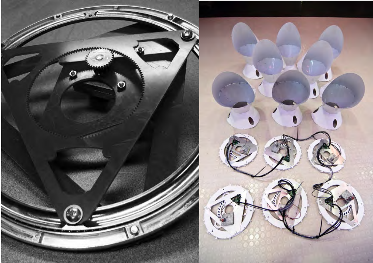
MacroBot & DeciBot internal gear, bearings, and communications.
