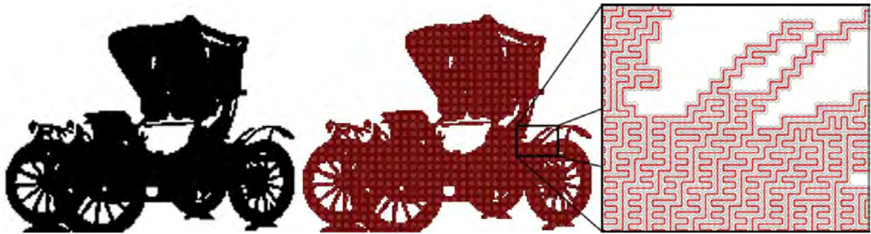
Automated path construction from an arbitrary shape.
