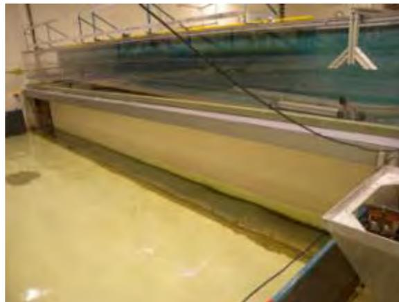
**Figure 5 Back view of the wavemaker used for wave generation in the wave basin**
