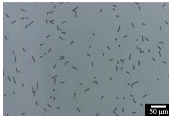
Fig. 4. Optical micrograph of glass rods dispersed in water in an anti-parallel rubbed cell.
