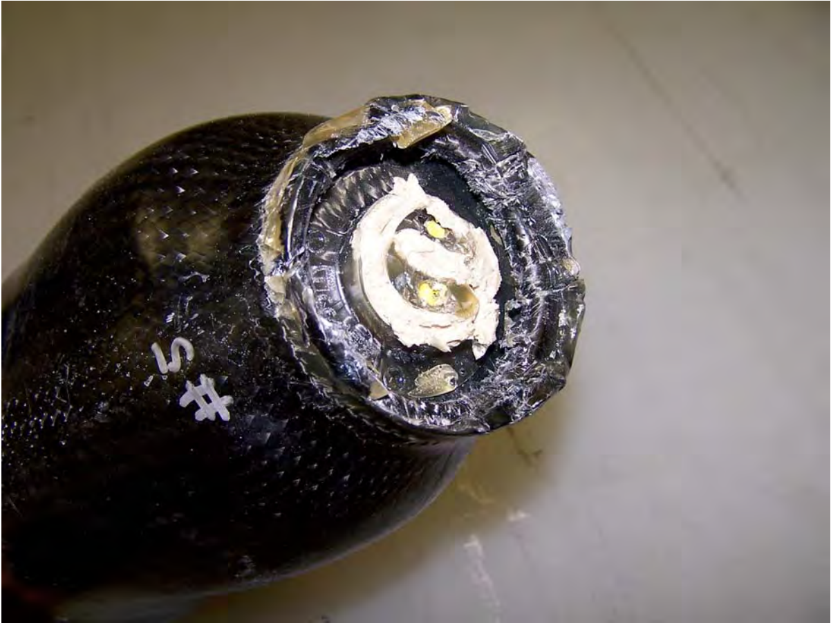
Figure 15. Failure region close-up view for socket #5.
