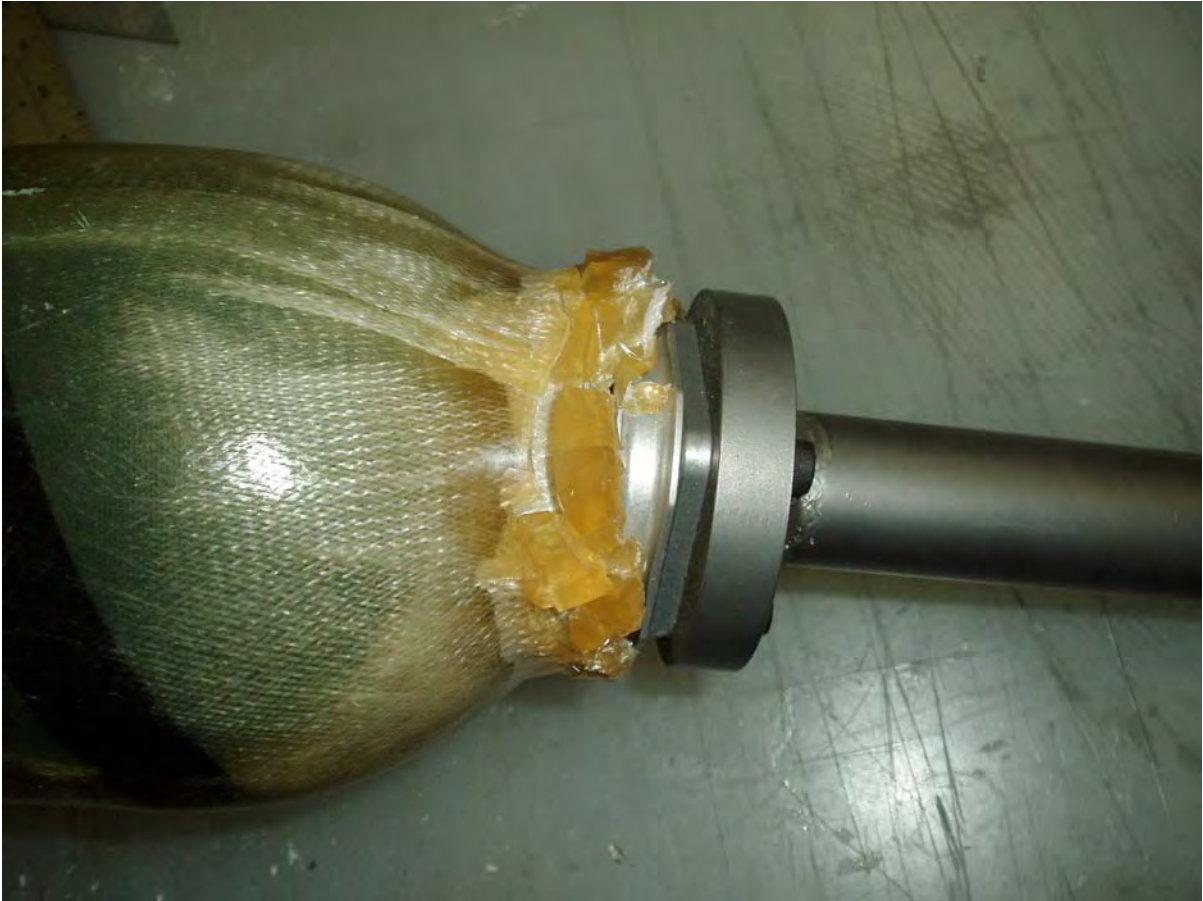
Figure 10. Failure region close-up view for socket #4.
