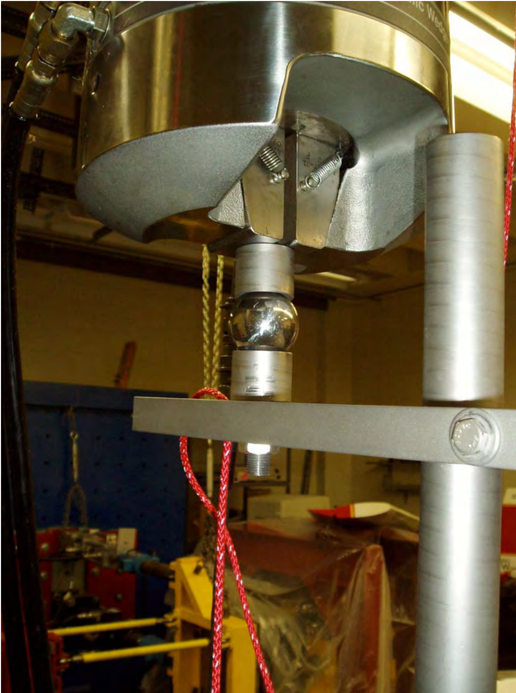
Figure 2. Distal end load fixture detail.
