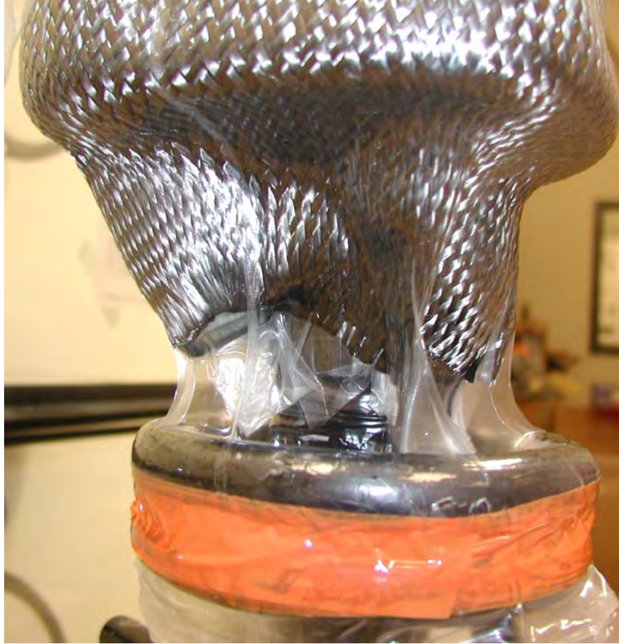
Figure 2: Illustration of the collapse of the vacuum bag
