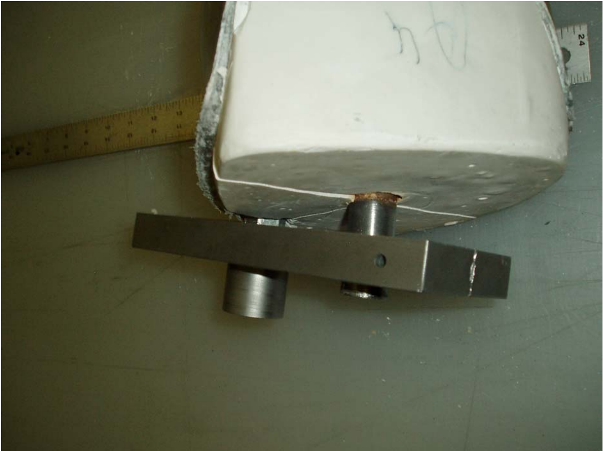
Figure 9. Steel shank plastic deformation and plaster mold cracking for socket #4.
