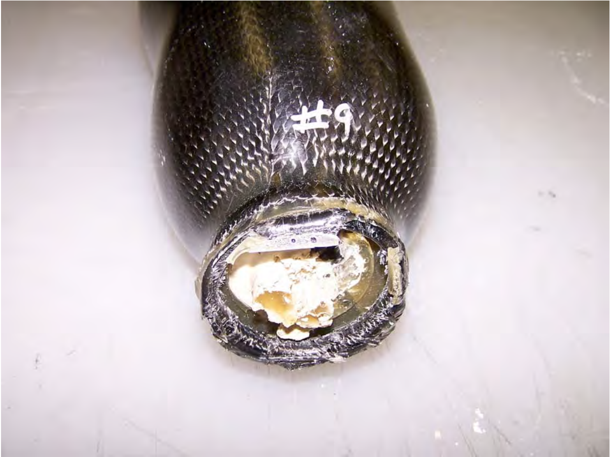
Figure 31. Failure region close-up view for socket #9.
