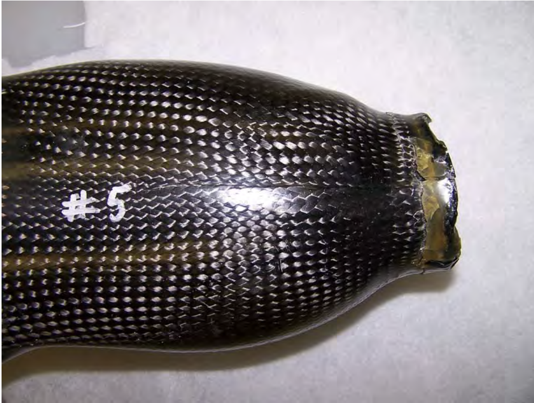
Figure 14: Medial close up of the failure of Socket #5
