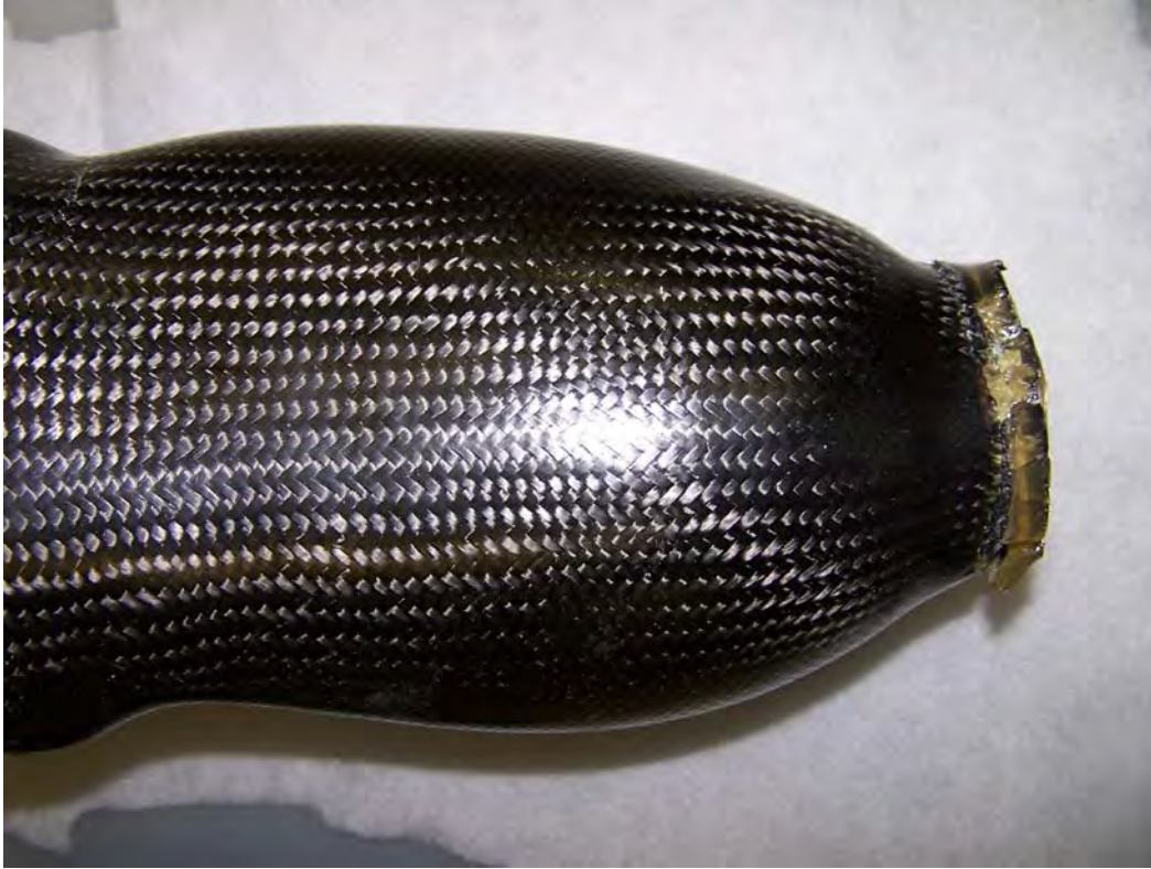
Figure 15: Medial close up of the failure of Socket #6
