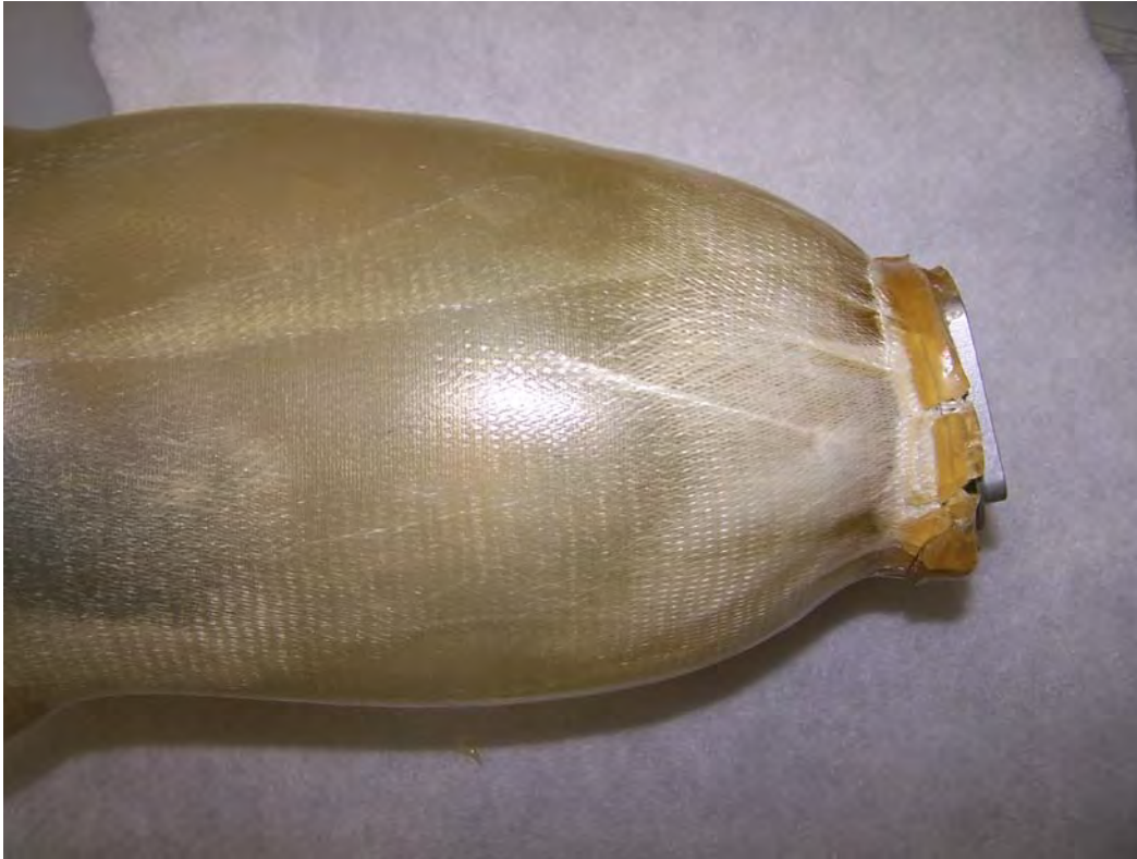
Figure 12: Medial close up of the failure of Socket #4
