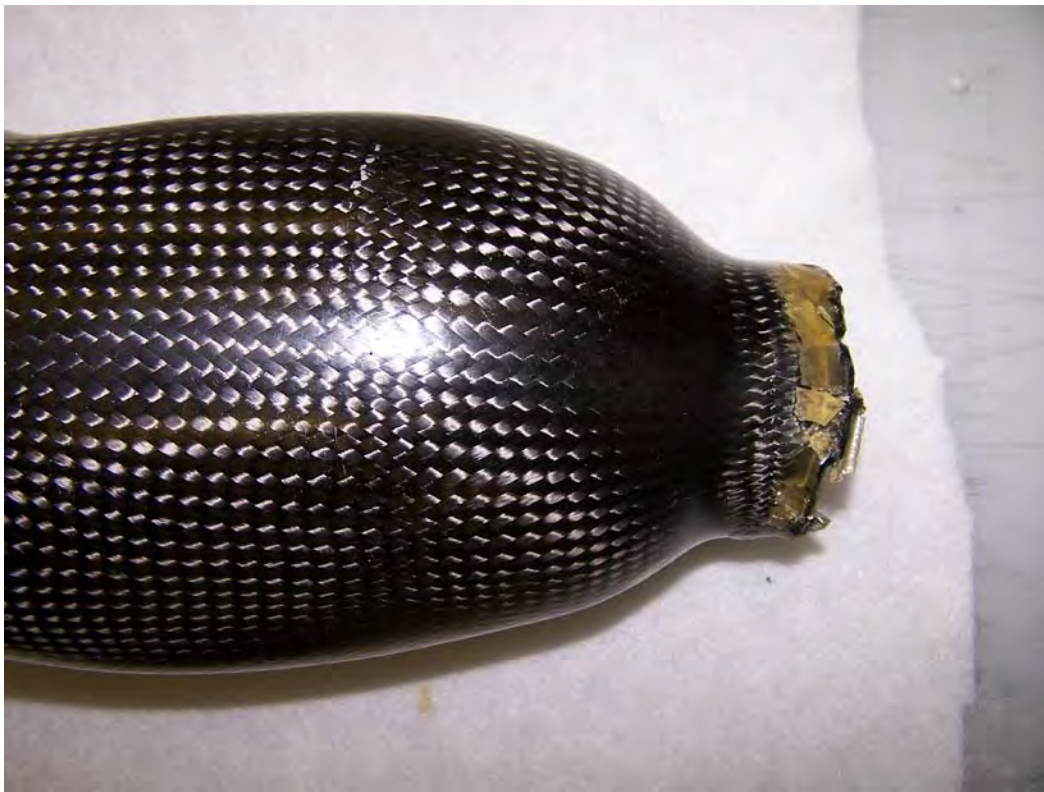
Figure 16: Lateral close up of failure of Socket #9
