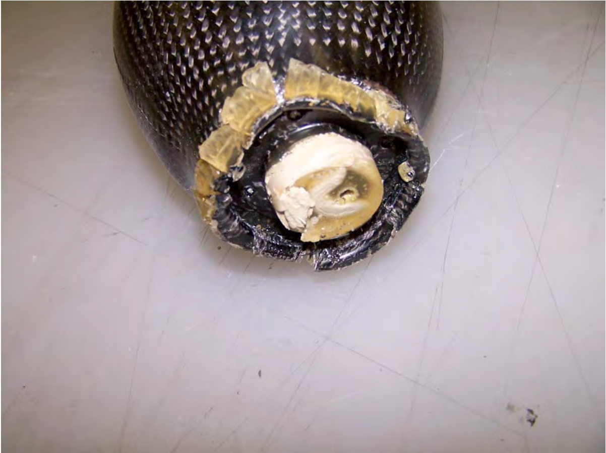
Figure 19. Failure region close-up view for socket #6.
