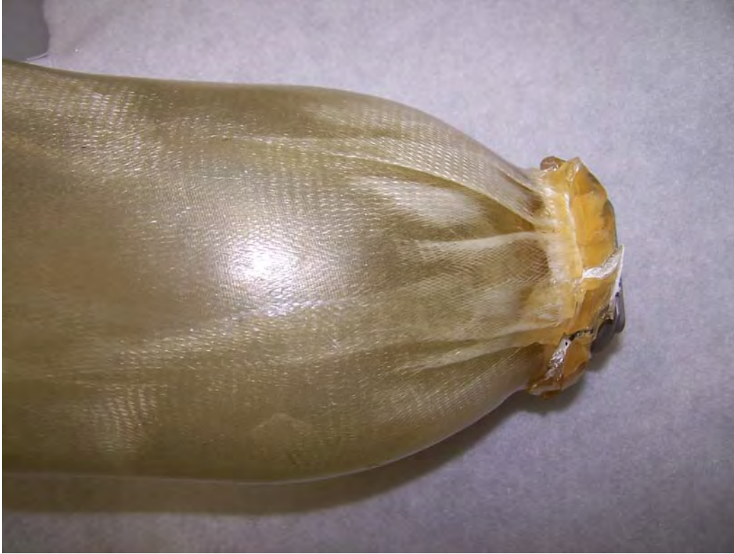
Figure 13: Posterior close up of failure of Socket #4
