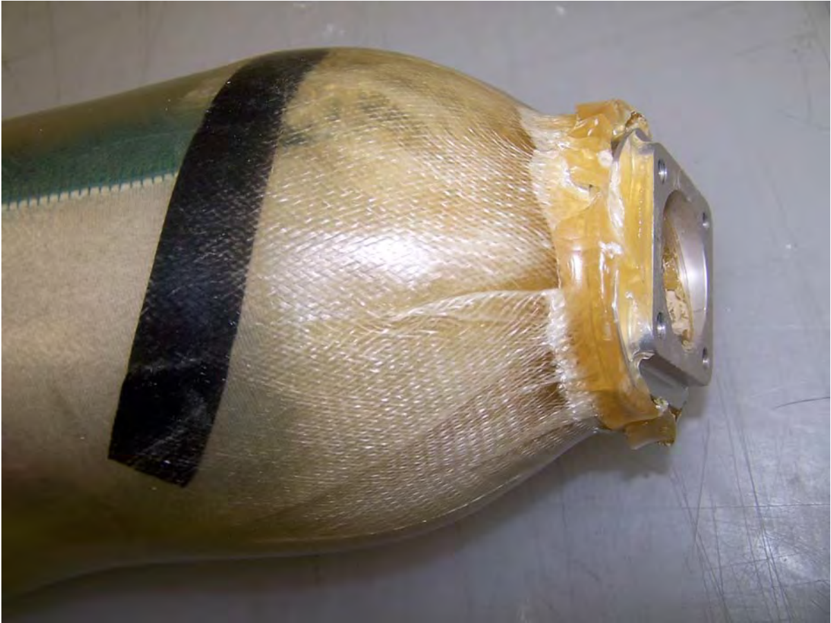
Figure 11. Failure region close-up view for socket #4.
