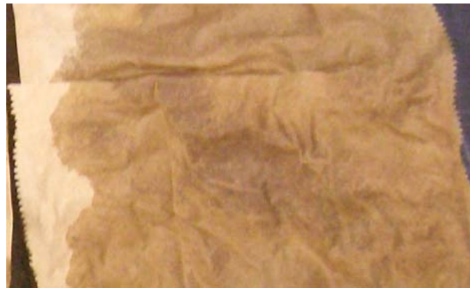
Figure 33. Cast cubes kept moist under paper towels.
