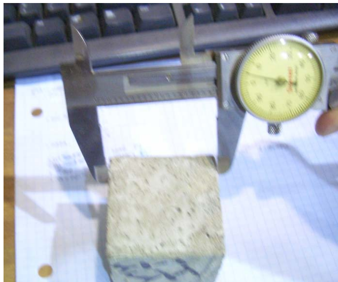
Figure 37. Determination of cube dimensions.
