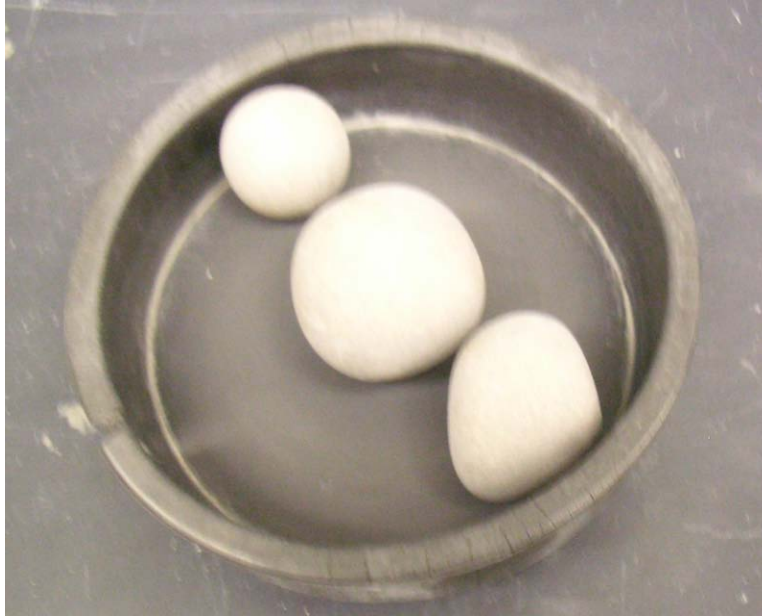
Figure 22. Typical stones used for mechanical crushing of pozzolan samples.
