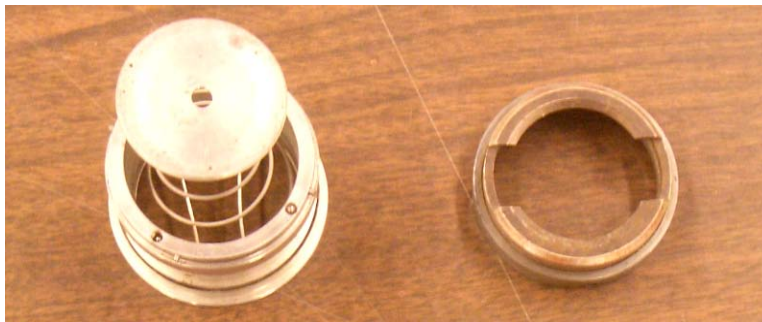
Figure 25. Spring and locking mechanism for the dish.
