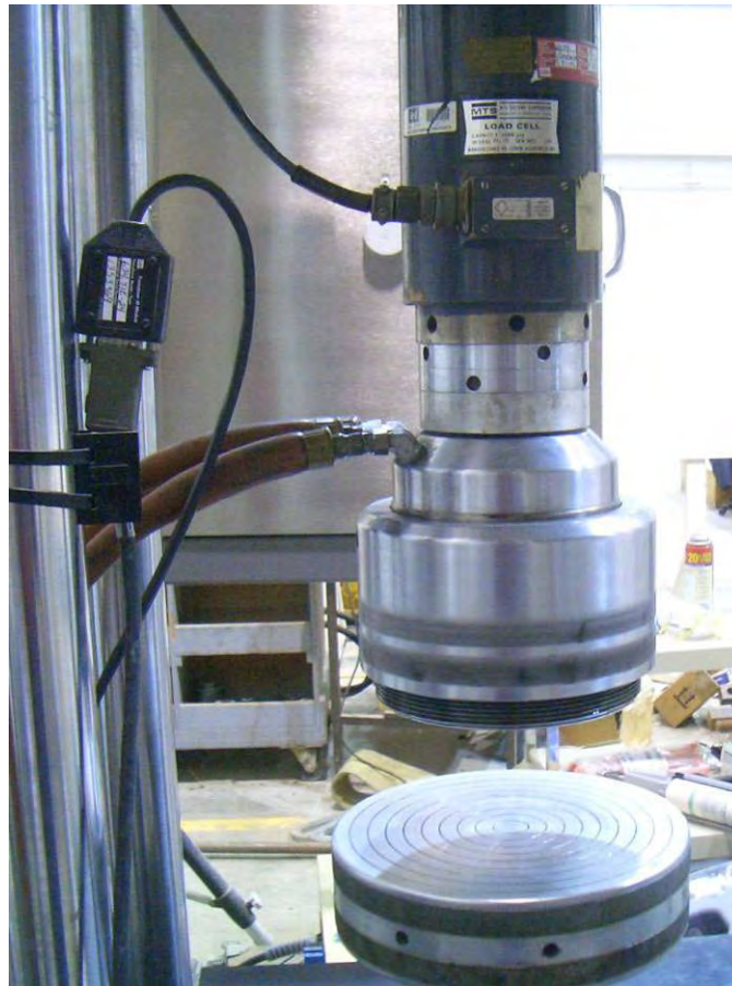
Figure 34. 50 kip loading machine.
