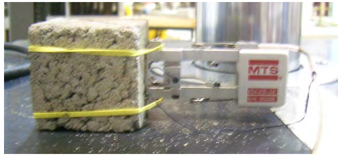
Figure 38. Extensometer attached to specimen.
