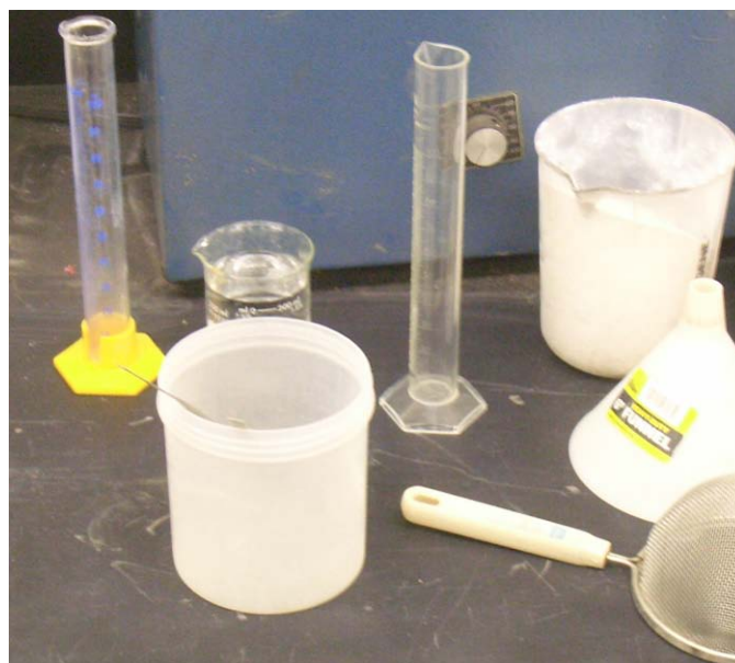
Figure 29. Measuring equipment for concrete mix.
