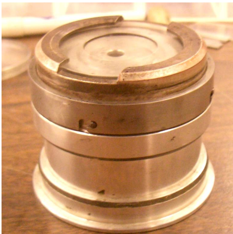
Figure 26. Assembled sample holder without sample loaded.
