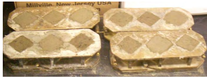
Figure 32. Concrete setting in cube molds.
