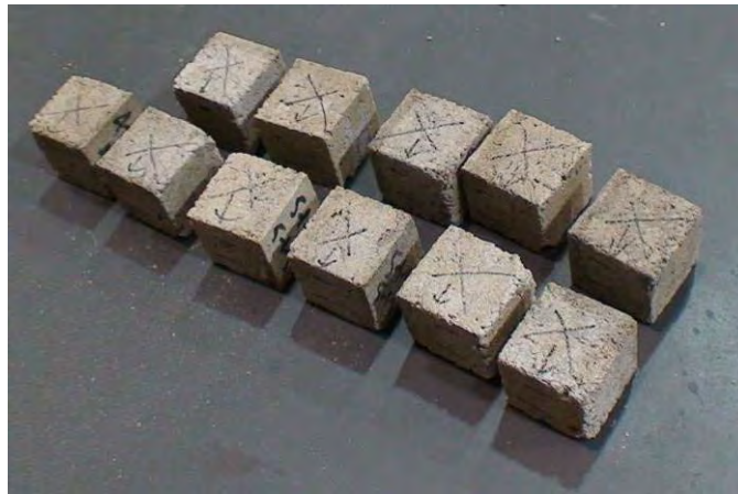
Figure 36. Cubes with faces to be compressed marked.
