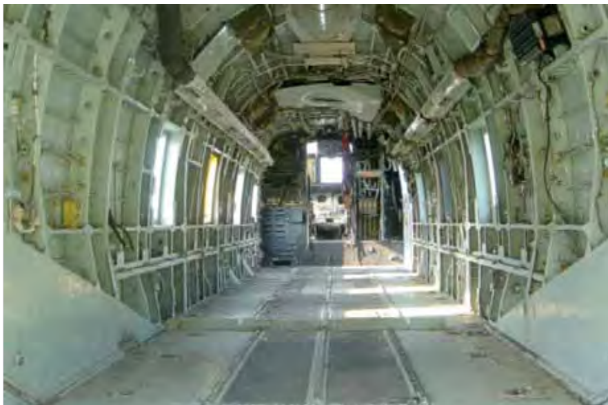
Figure 3 HH-3 Fuselage Interior
