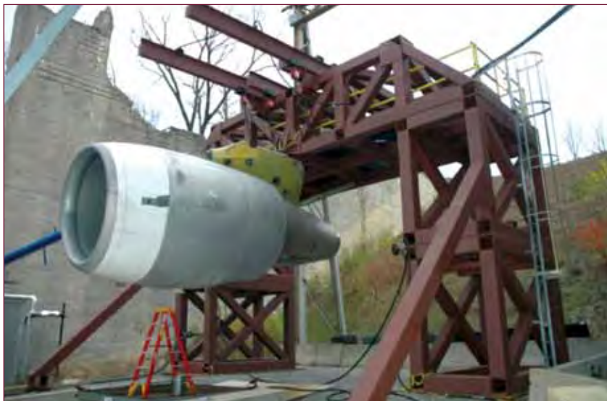
Figure 2 CF6-50 Engine Mounted on Test Stand
