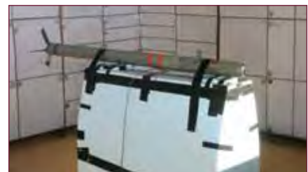
Figure 3 Missile Positioned in the Center of the Static Test Arena
