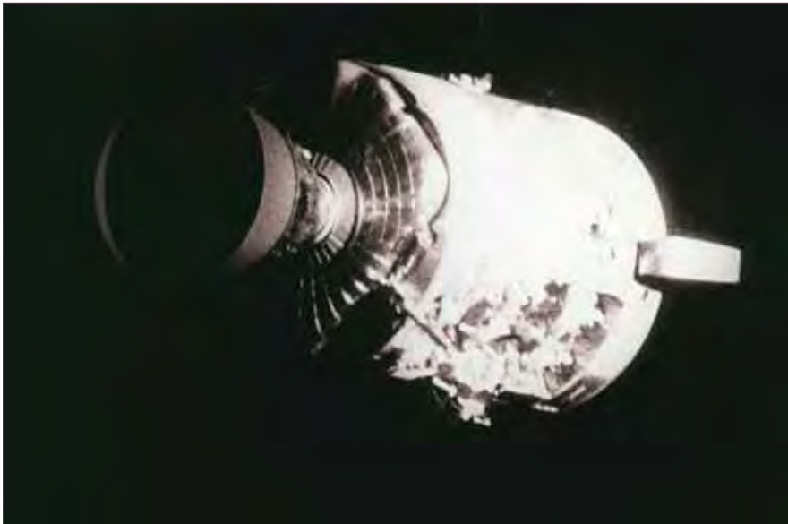
Figure 6 An entire panel of the Apollo 13 service module was blown away by the apparent explosion of oxygen tank number two, located in sector 4 of the SM. Two of the three fuel cells are visible just forward of the heavily damaged area.
