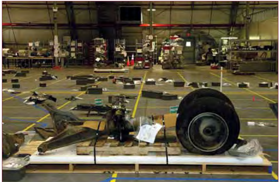
Figure 5 Among the larger pieces of debris recovered from the crash of Columbia was its nose gear, shown here with its tires still intact.
