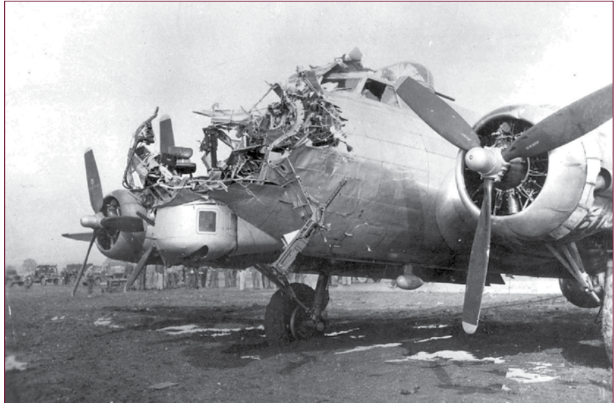
Figure 1 Flak damage completely destroyed the nose section of this Boeing B-17G, A 398th Bomb Group aircraft flown by 1Lt. Lawrence M. Delancey over Cologne, Germany. USAF photo
