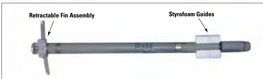
Figure 1 Example Missile Configuration for Gas-Gun Launch
