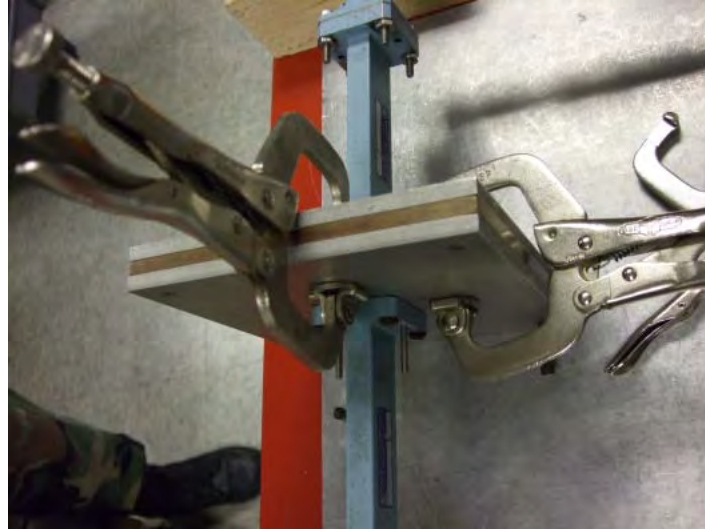
Figure 29: Short measurement with the brass plate between the two mounting plates
