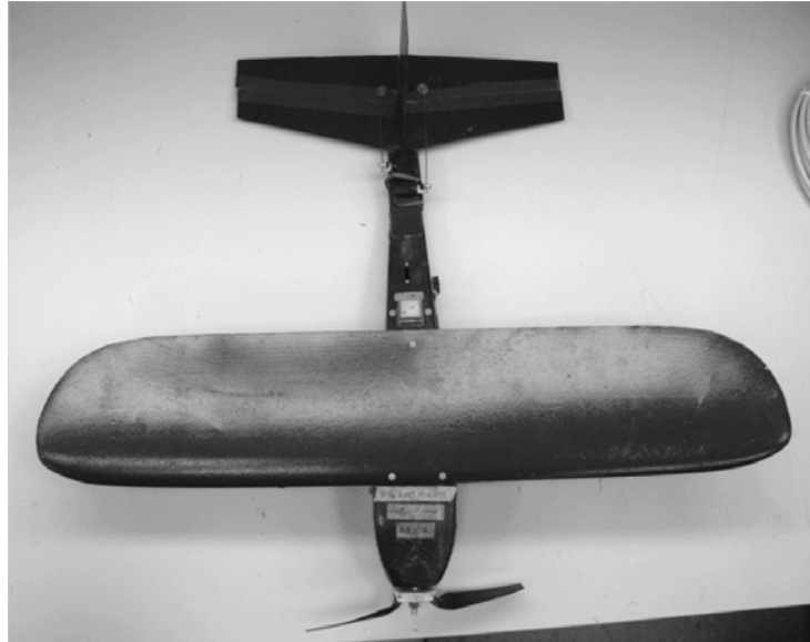
Figure 3. GENMAV SUAS developed by AFRL (Abate, Stewart and Babcock 2009)
