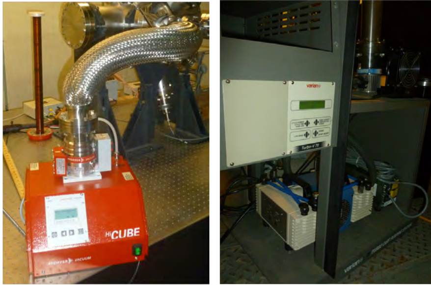
Figure 19. Pictures of the Pheiffer HiCube 80 Eco turbo pumping station (left), Varian V-70LP turbo pumping station (right), connecting hardware, and the MDC vacuum chamber.
