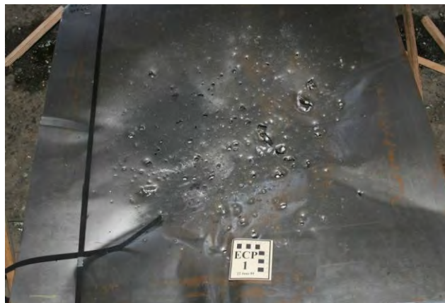
Figure 6. Witness plate after being hit with spall generated from the testing process.
