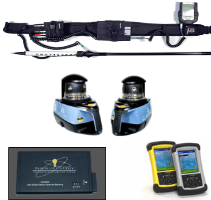
Figure 1. iGPS unit used by TMT to capture reference points. Points are collected through the tip of the arm shown at the top.
