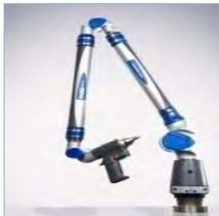
Figure 2. Scanning arm used to collect point data and capture curves.
