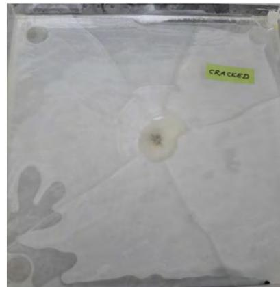
3b Top View of a damaged Armor Sample
