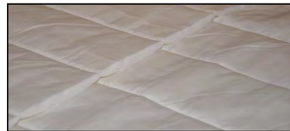
Manufacturing Quilt Lines of Current Prototype Liner System
