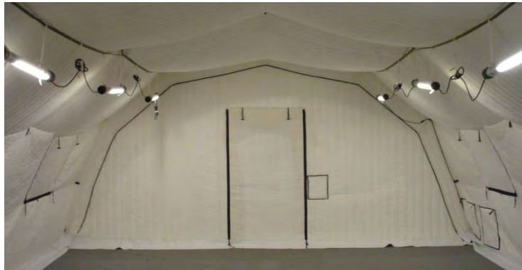
Airbeam Shelter with a Prototype Non-woven Insulation Liner
