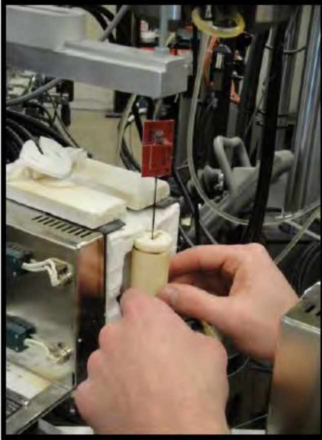
Figure 40 : Assembling the susceptor with the specimen passing through the upper and lower plates.
