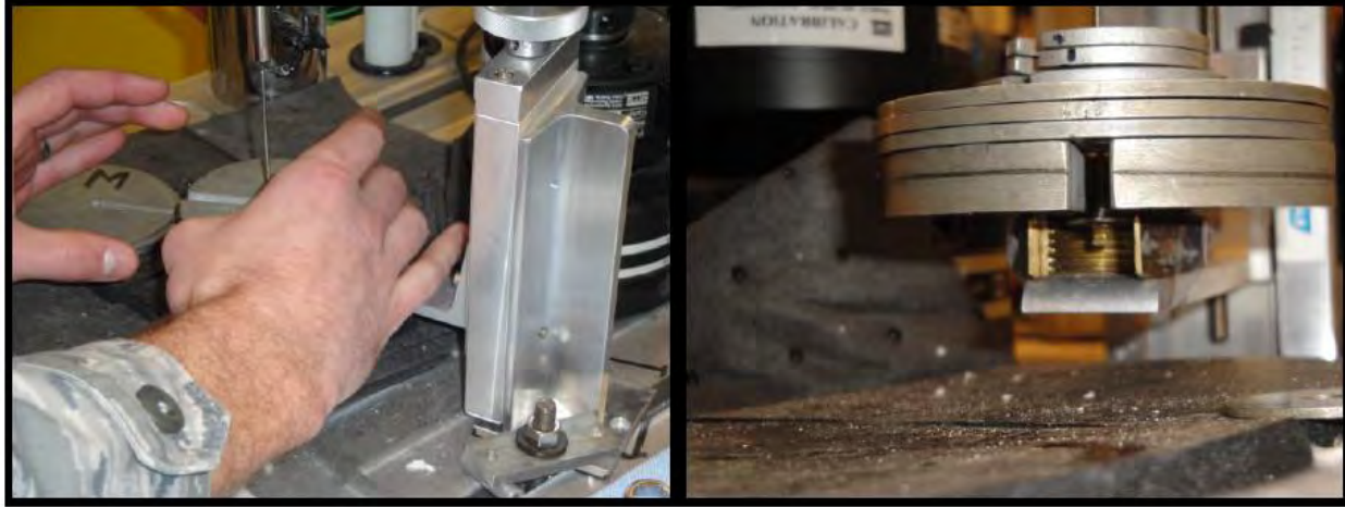
Figure 37 : Stacking the weights onto the split-nut and load train staged in weight stack.
