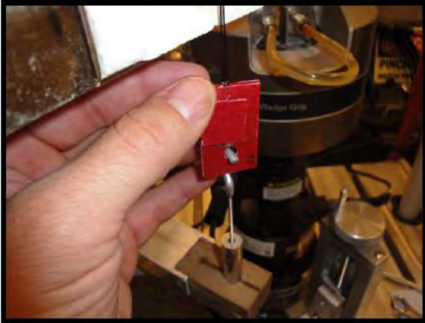
Figure 39 : Installing the Hi-Nicalon S fiber tow specimen onto the lower hook.
