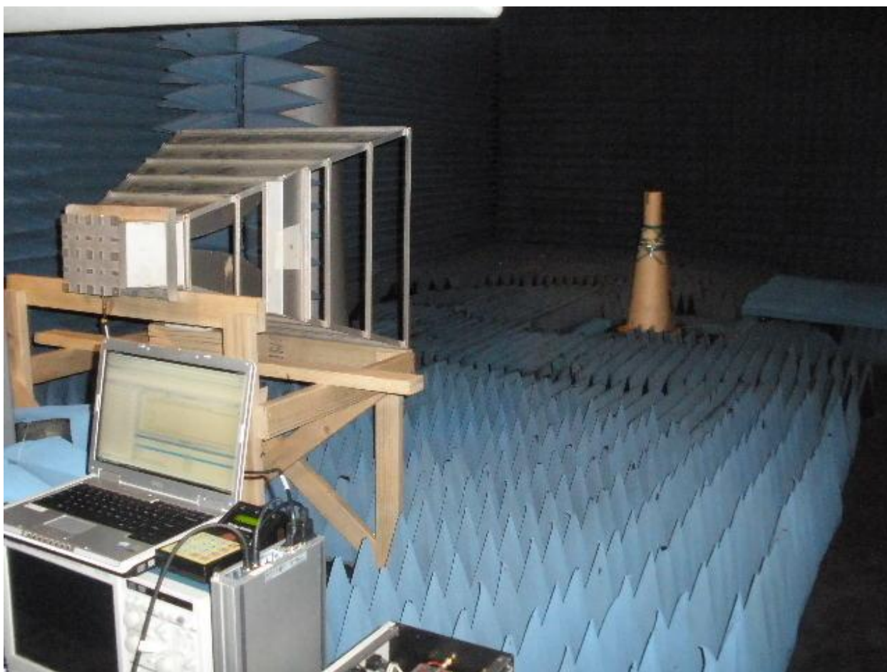
Figure 44 – Full anechoic chamber setup
