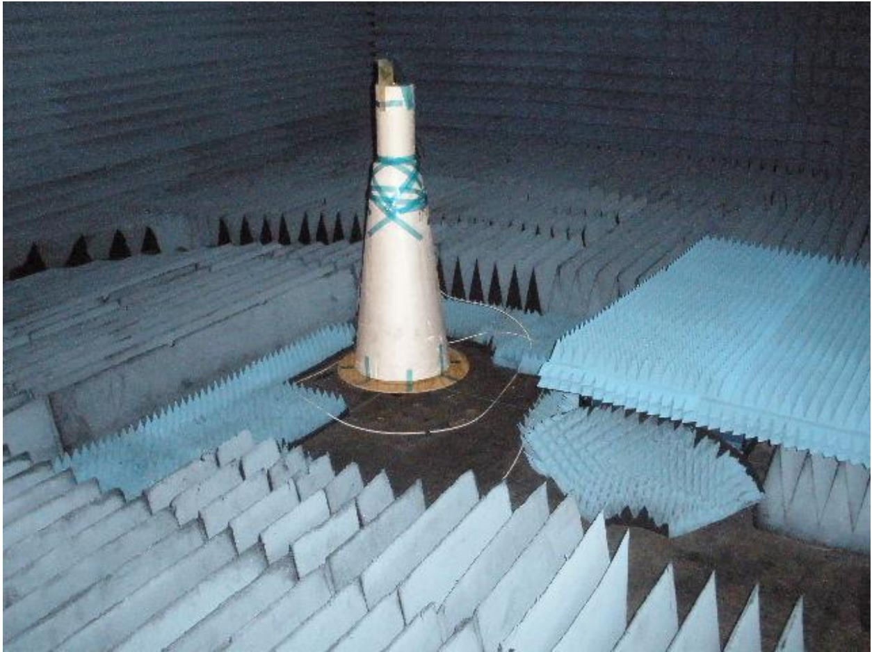
Figure 45 – AUT pylon setup on stepper motor rotating platform
