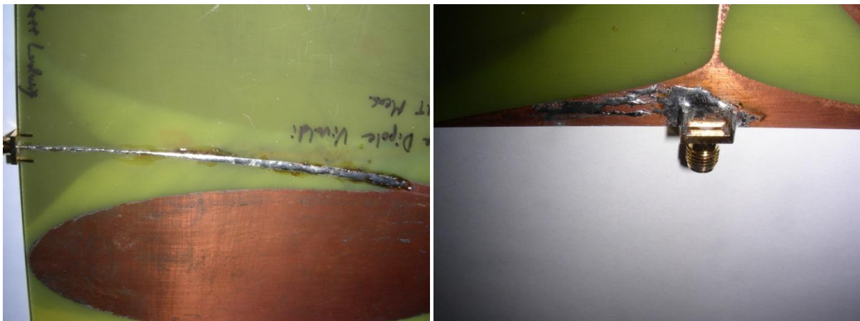
Figure 41 – Soldering fix to gaps left by PCB etching process
