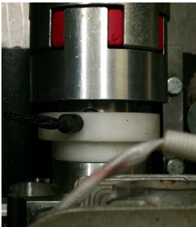
Figure 34: Brison Hall-Effect sensor
