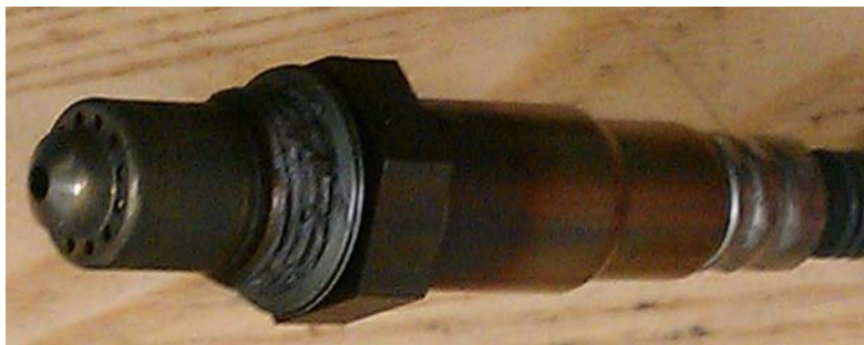
Figure 31: Bosch LSU 4.9 oxygen sensor
