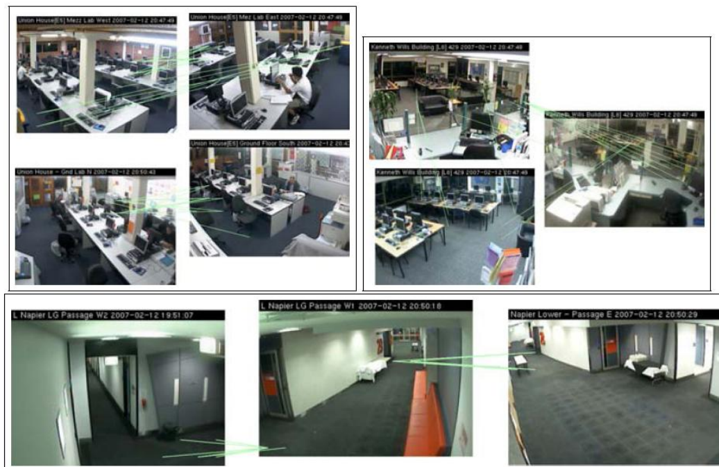
Figure 2: Groups of images whose views are overlapping. The edges of the vision graph are shown in green.
