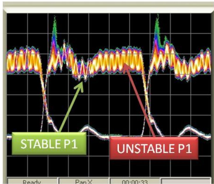
Figure 4.18: Eye diagram of communication signal with region of stable and unstable P1 frequency in the same symbol.
