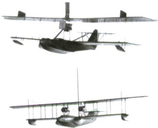
Figure 16. Most of the Navy's flying boats were tested in the Navy's wind tunnel including the HS-1 (top) and H-12 (bottom) aircraft.
