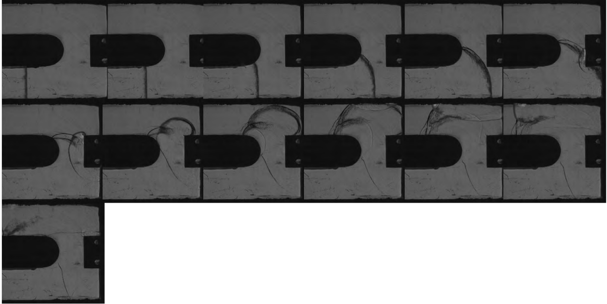
Figure B-11. Hydrogen-air detonation in mid-mid configuration with 1.5 in crossover width resulting in a successful Region III reinitiation
