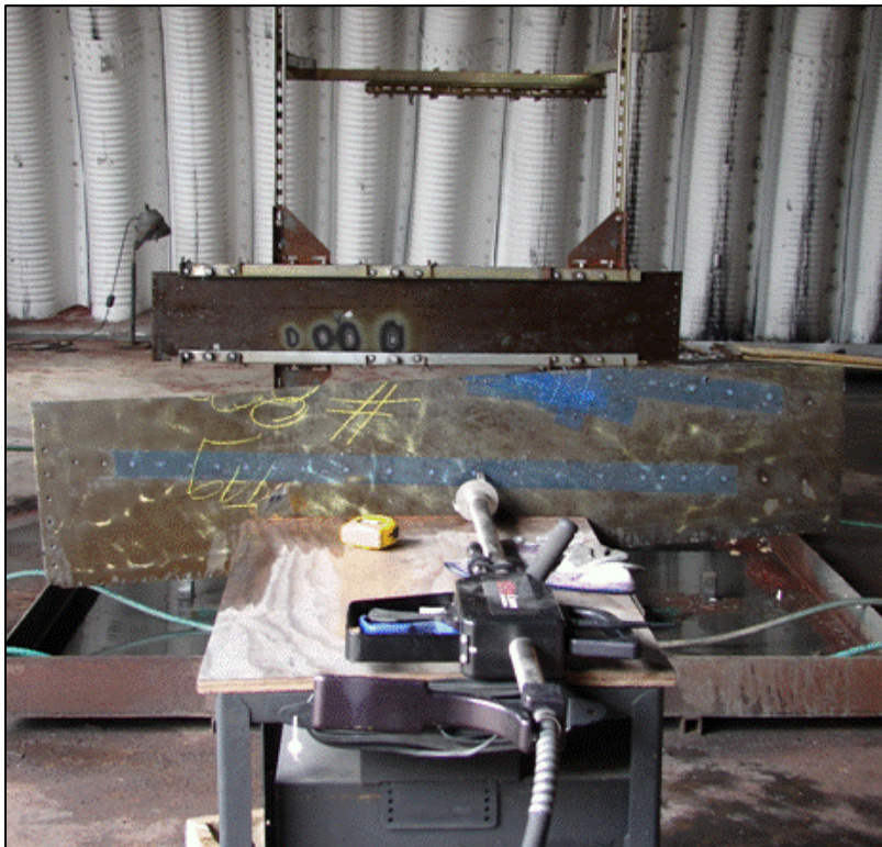
Figure 24. Setup for Two Composite Panel Penetration Evaluations
