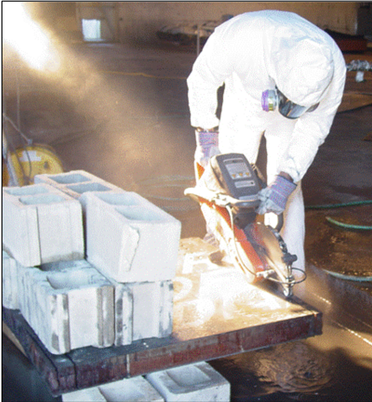
Figure 11. Cutting B-2 Composite Door Using Circular Saw
