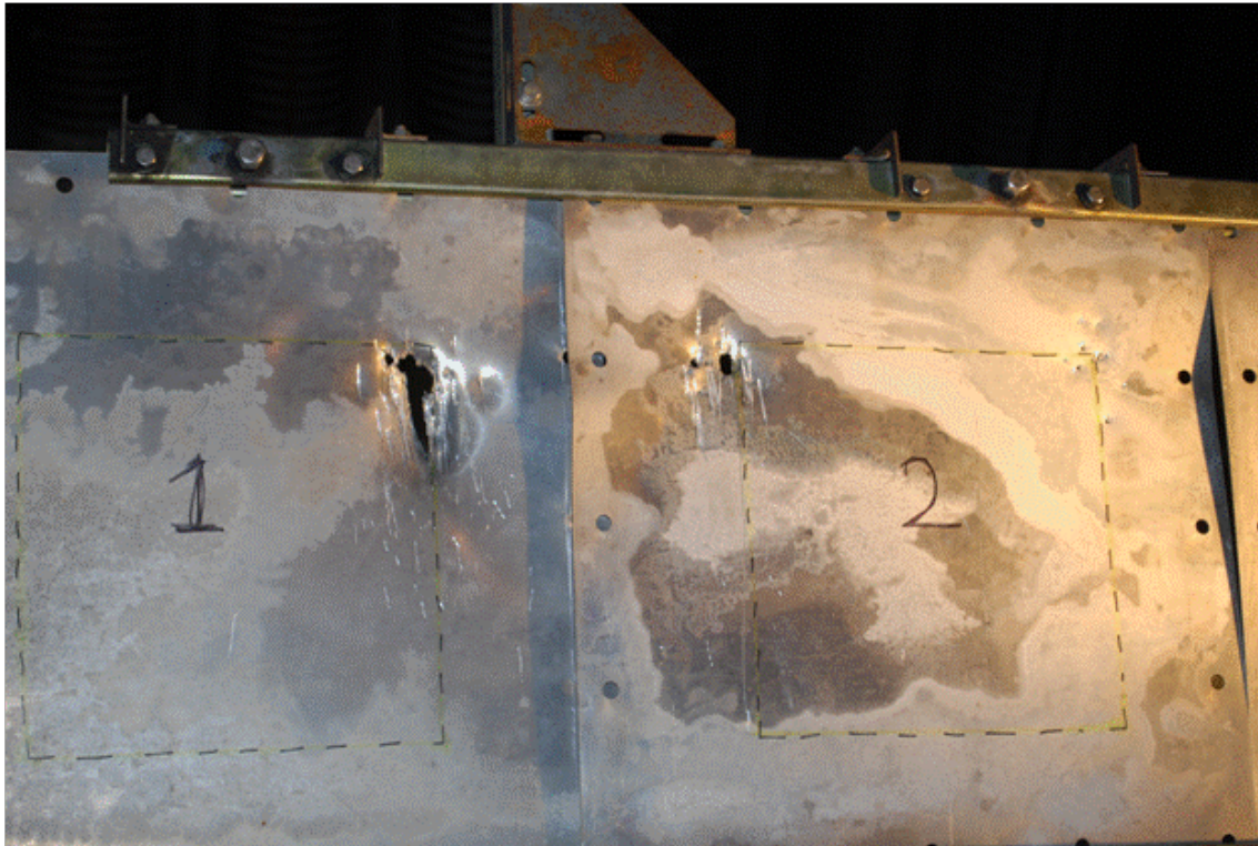
Figure 19. Pry Axe Used on 5052-H32 Aircraft Aluminum
