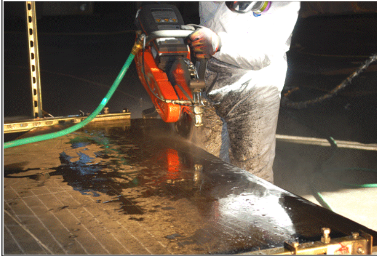
Figure 10. Circular Saw Being Used to Cut F-16 Composite Sheets
