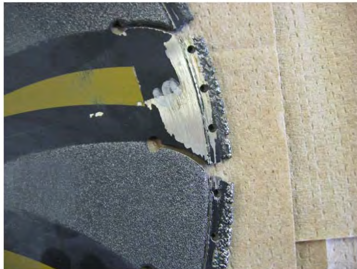
Figure 3: Circular Saw NDL 18772 no. 2, after testing
