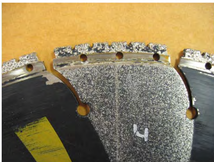
Figure 6: Circular Saw NDL 18772 after third round of testing
