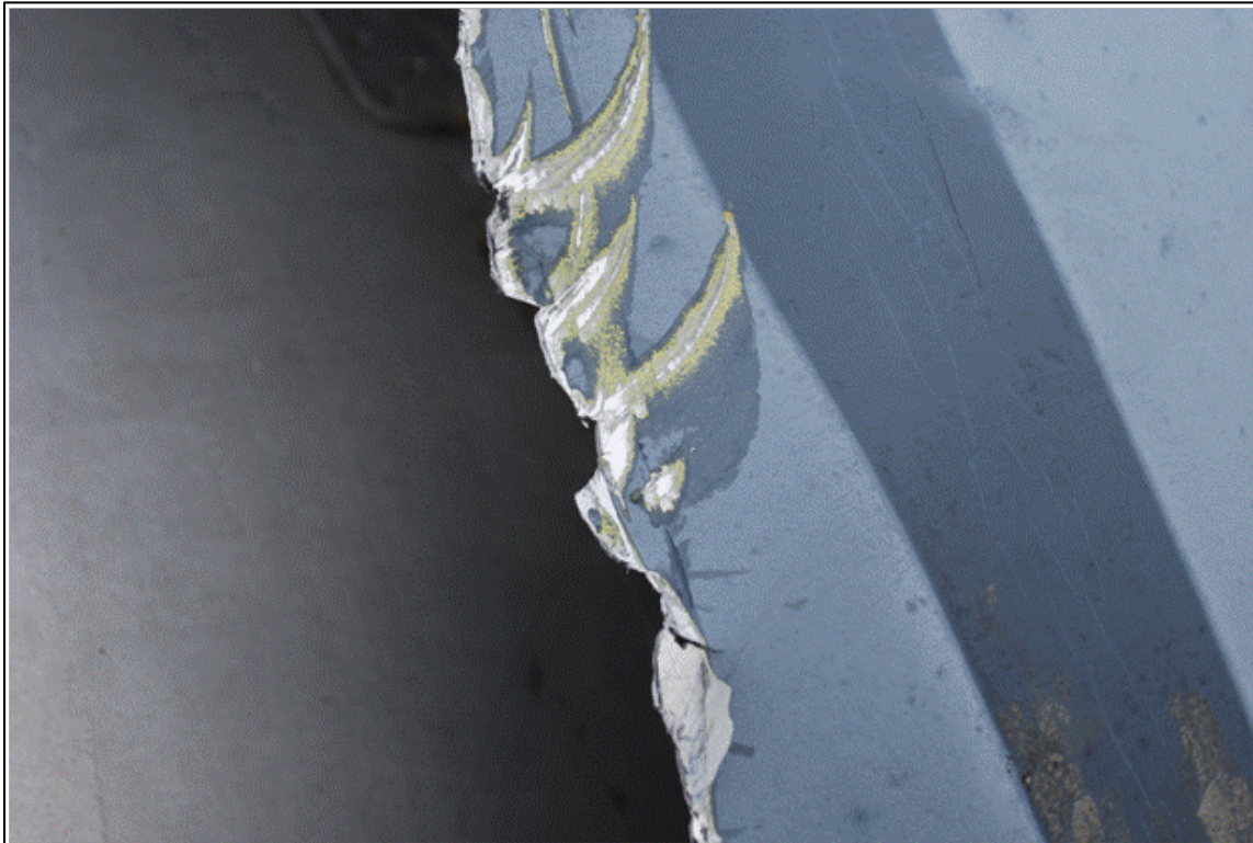
Figure 22. Edges of KC-135 Engine Nacelle Cowling after Cutting with Pry Axe
