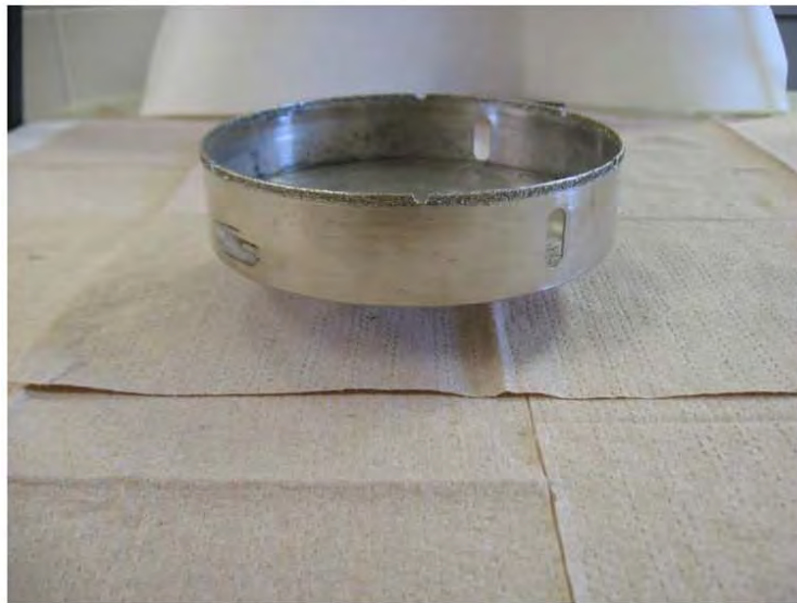
Figure 11: Hole Saw 152 mm after testing
