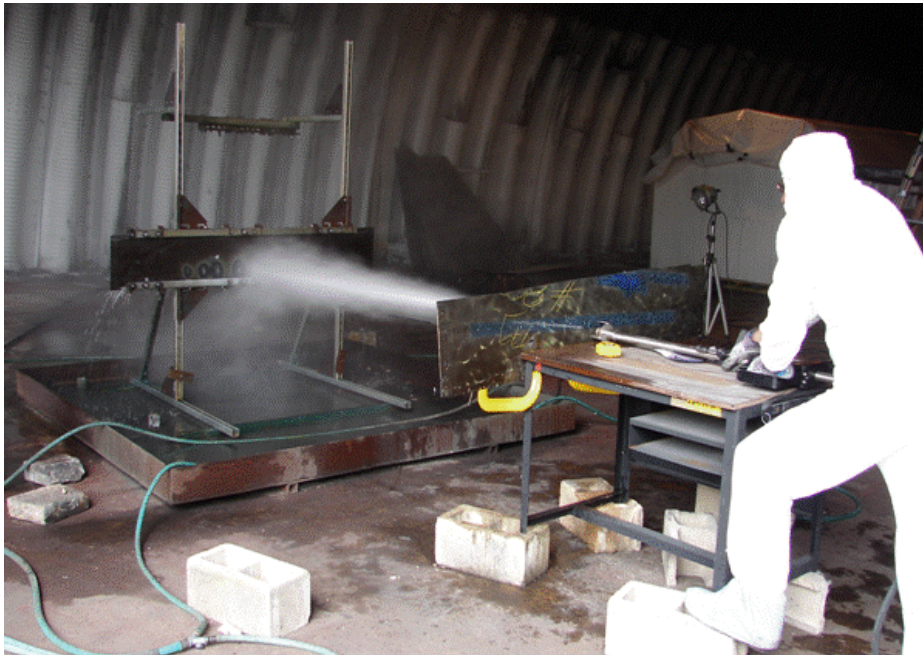
Figure 29. Testing the Effective Piercing Distance of Pyrolance
