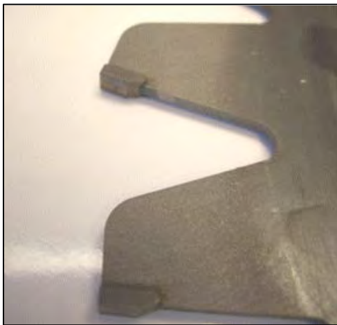
Figure 6. Close-Up of Carbide (left) and Diamond (right) Circular Saw Blades before Cutting
