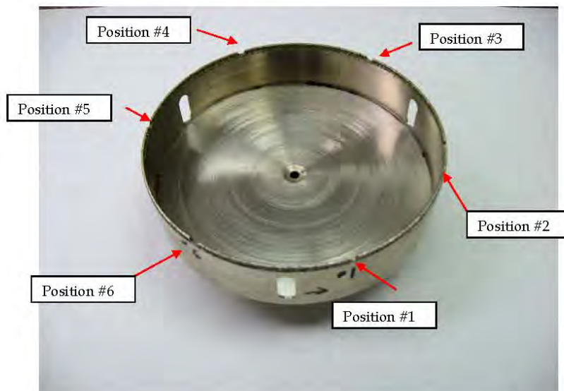
Figure 3: Macrograph of Hole Saw 152 mm before testing, showing position locations
