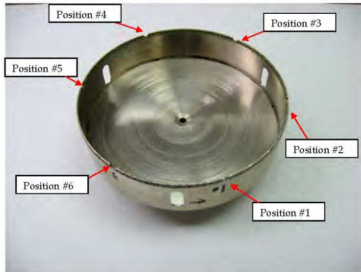
Figure 9: Macrograph of Hole Saw 152 mm before testing, showing position locations
