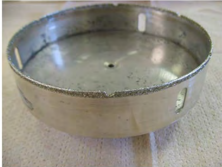
Figure 10: Hole Saw 152 mm after testing
