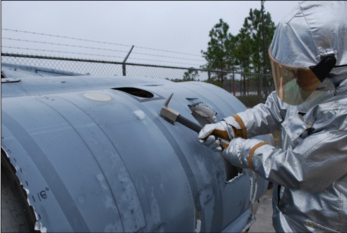
Figure 21. Demonstration of Pry Axe Cutting Access Hole in KC-135 Engine Nacelle Cowling
