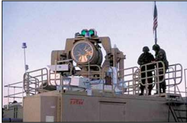
Figure 6. Tactical High-Energy Laser (THEL)
