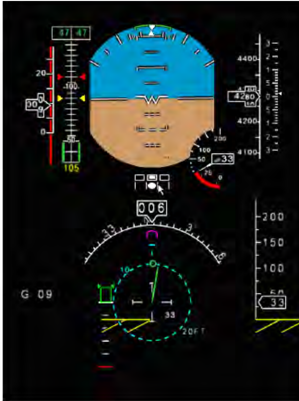
Figure A-11a): CAAS Display Modified with an Integrated Altimeter and Vertical Speed Indicator.
