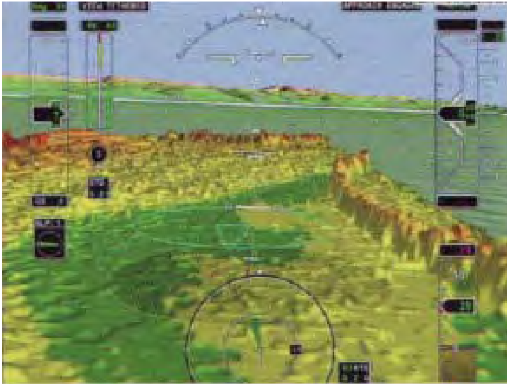
Figure A-7: Sandblaster Display Includes Radar Data (Close) and Pre-Stored Terrain Elevation Data (Far) and Symbology.
