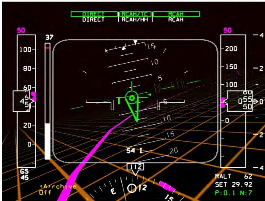
Figure A-3: New Flight Path Marker Symbol (ATP-FPM) Used with Synthetic Terrain Imagery as Flown on the US Army Fly-by-Wire RASCAL UH-60.
