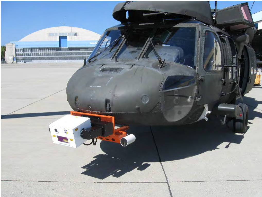
Figure C-1: Gimbaled LADAR, Fixed FLIR, and Fixed Color Camera Mounted on Aircraft Nose.
