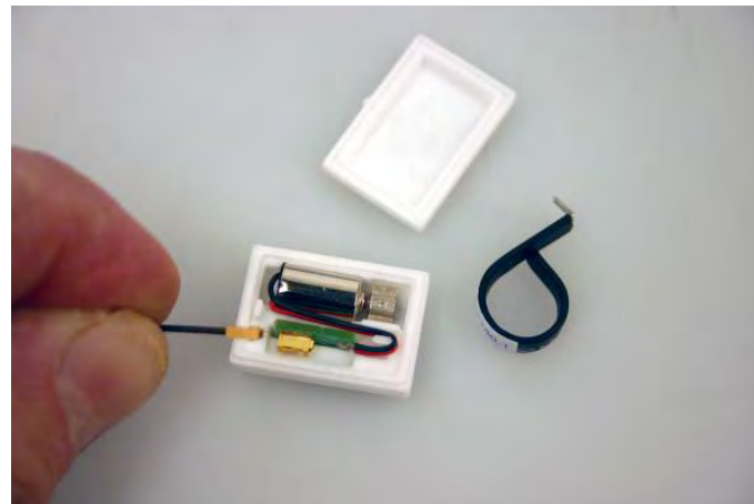
Figure B-3: TNO Tactile Torso Display (Left) and Inside View of a Tactor (Right).
