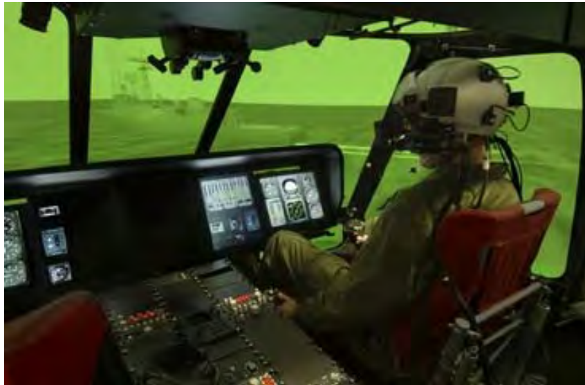
Figure A-31: AS Simulation of Seahawk Operating to FFG Frigate with NVGs and HUD.
