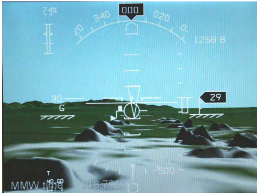
Figure A-17: BAE Terrain Elevation Data Morphed with Simulated Radar Data.
