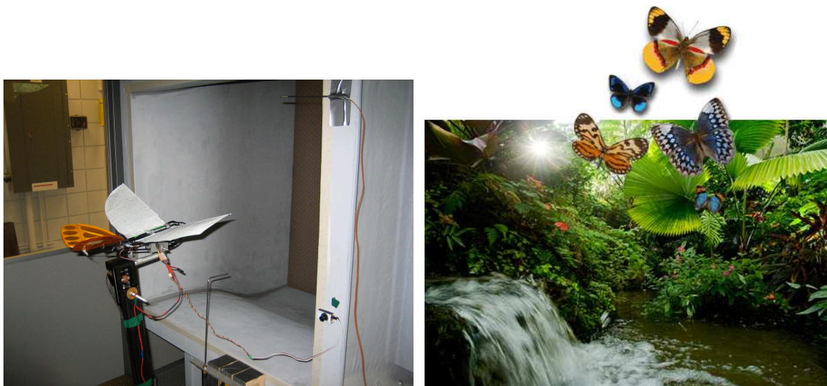
Figure 1. (a) A 20 cm wingspan ornithopter with a flexible wing in the REEF small wind tunnel. (b) The rain forest at the McGuire Center for Lepidoptera and Biodiversity, Gainesville, FL.
