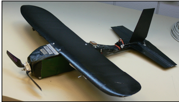
Figure 2. Attitude control demonstrations were based on a model of the AFRL GenMAV vehicle. Aerodynamic coefficients were calculated using AVL. Models assumed a configuration with ailerons, not shown in the hardware depicted.
