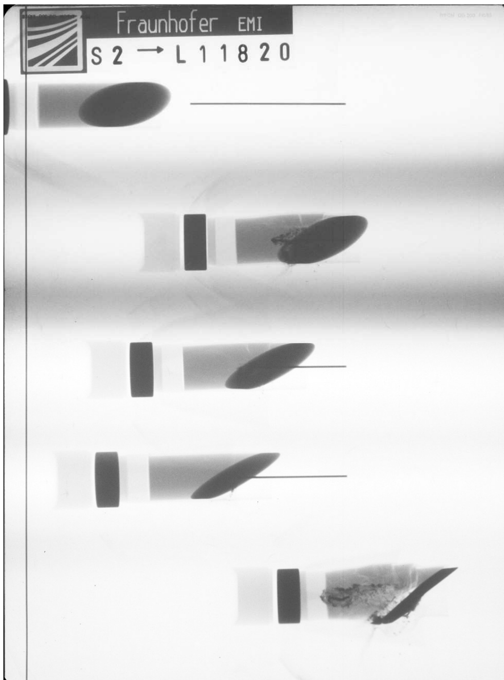
Figure A-63. X-ray picture for Exp. 11820: 60° with buffer, v_p = 1.613 km/s.
