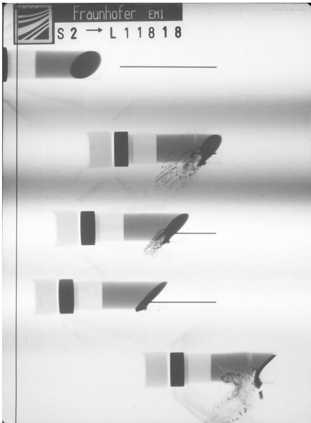
Figure A-33. X-ray picture for Exp. 11818: 45^\circ with buffer, v_p = 1.593 km/s.
