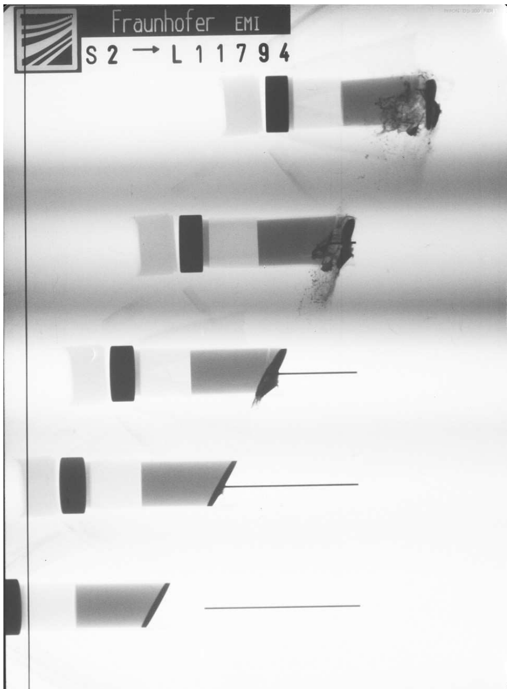
Figure A-13. X-ray picture for Exp. 11794: 30° with buffer, v_p = 1.529 km/s.
