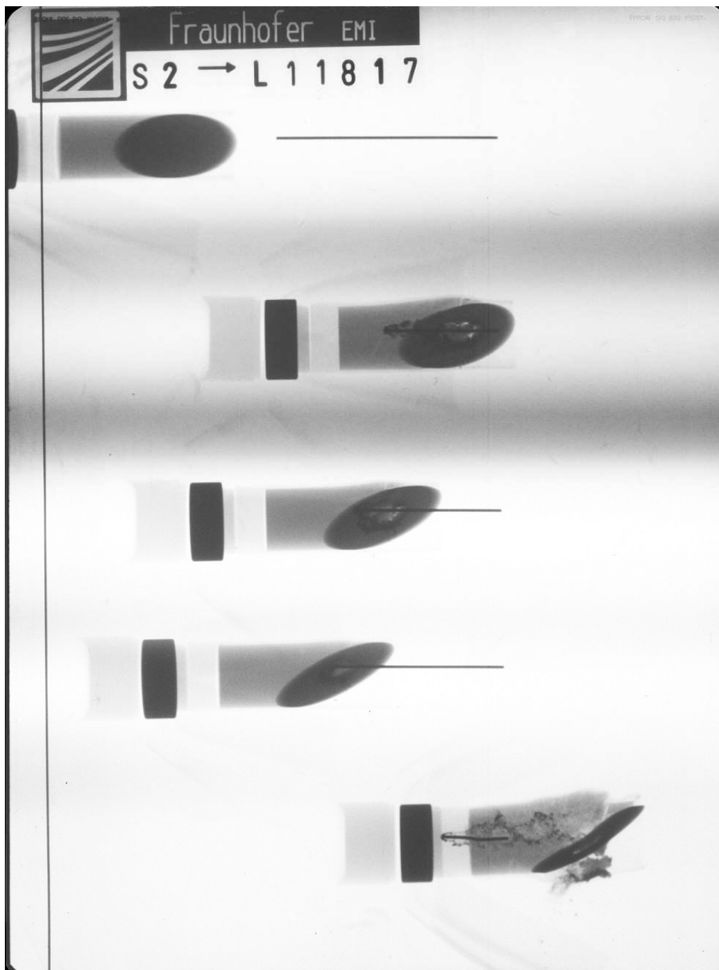
Figure A-61. X-ray picture for Exp. 11817: 60° with buffer, v_p = 1.569 km/s.
