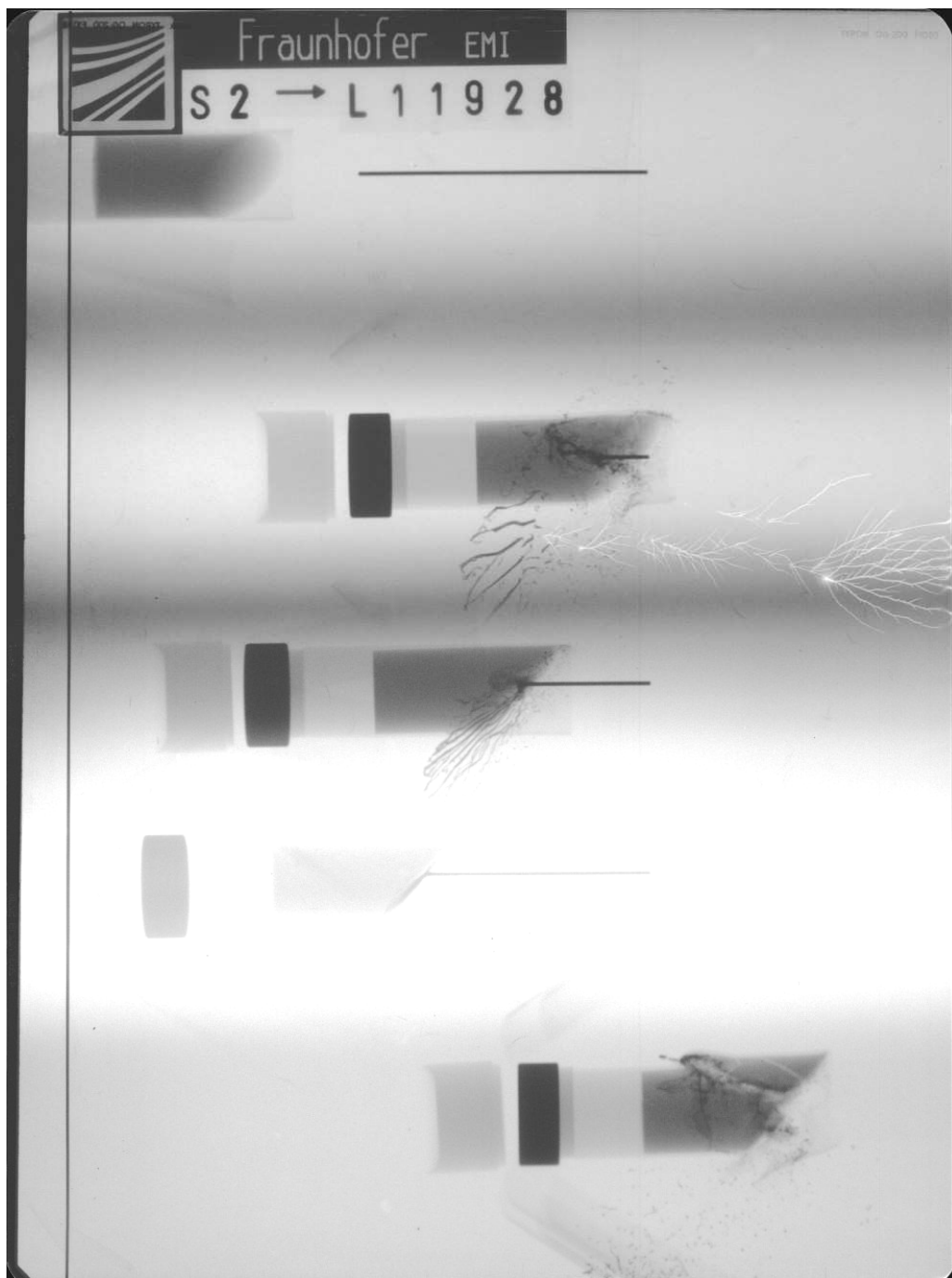
Figure A-37. X-ray picture for Exp. 11928: 45° bare, v_p = 1.015 km/s.
