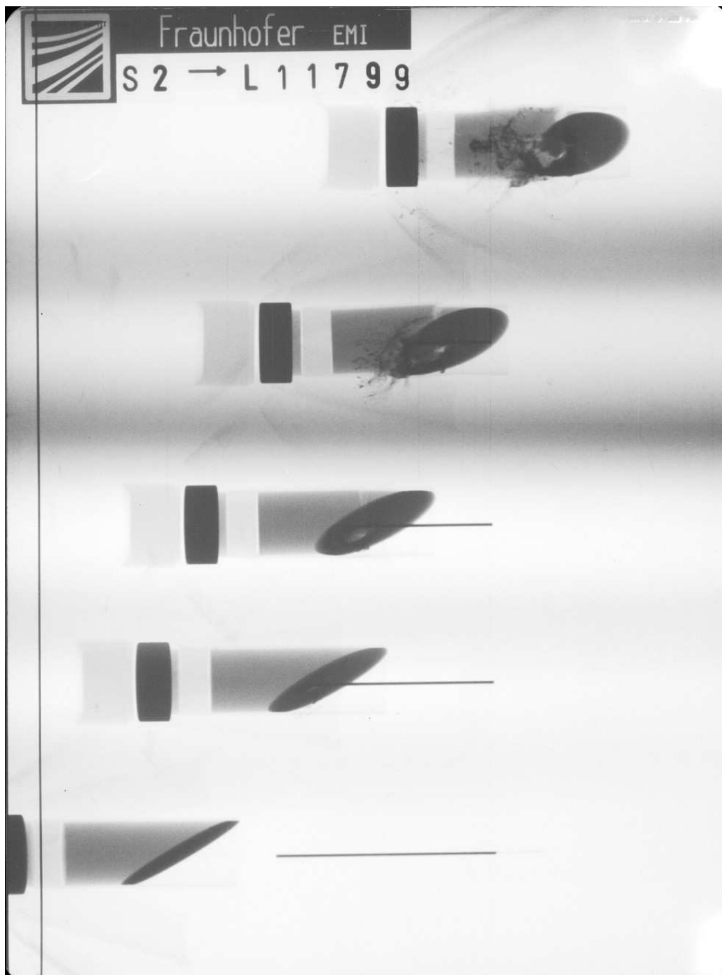
Figure A-59. X-ray picture for Exp. 11799: 60^\circ with buffer, v_p = 1.570 km/s.
