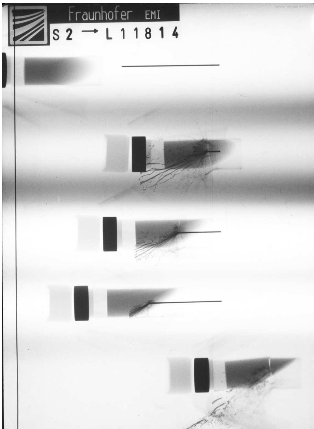
Figure A-75. X-ray picture for Exp. 11814: 60° bare, v_p = 1.408 km/s.
