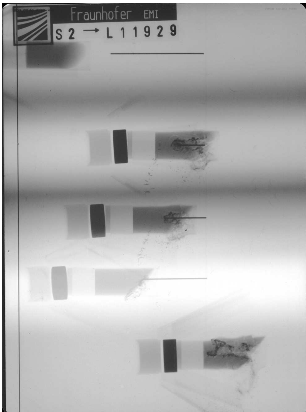
Figure A-45. X-ray picture for Exp. 11929: 45° bare, v_p = 1.191 km/s.
