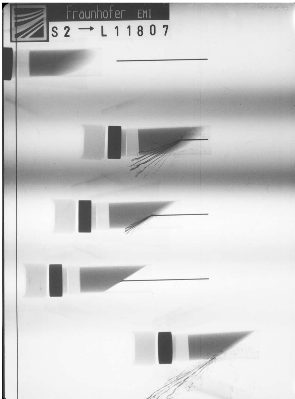
Figure A-65. X-ray picture for Exp. 11807: 60° bare, v_p = 0.921 km/s.
