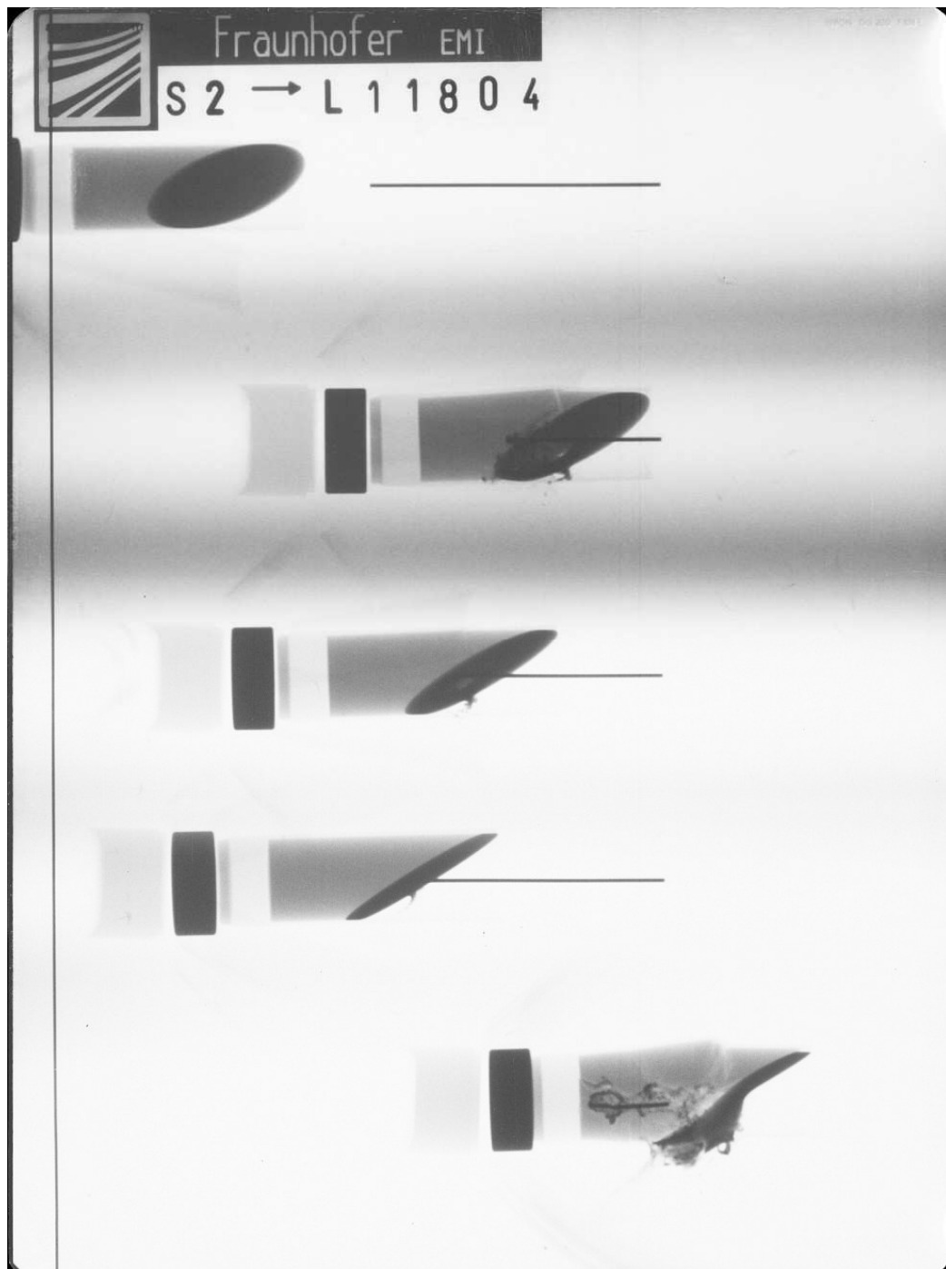
Figure A-51. X-ray picture for Exp. 11804: 60^\circ with buffer, v_p = 1.497 km/s.
