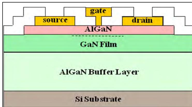
Figure 17. Schematic of a GaN/AlGaN HEMT structure grown on Si.
