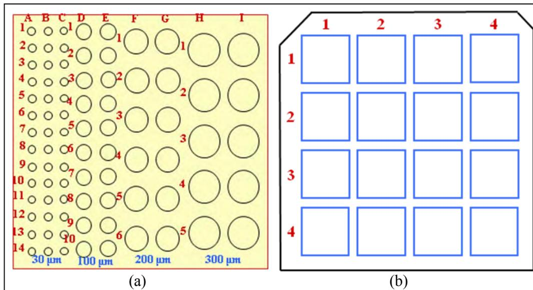
Figure 4. (a) Layout of the diodes in a unit cell and (b) layout of the cells on  $\sim 1 \text{ cm} \times 1 \text{ cm}$  wafer.
