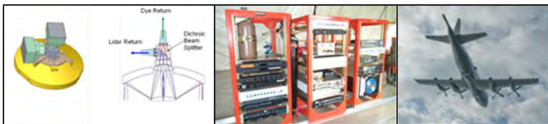
Figure 1 (l) Drawing of telescope redesign to record simultaneous backscatter and fluorescence signals; (c) interior picture of system install on P3, (r) belly window visible, lidar telescope and scanner are located above window, under floor of P3.
