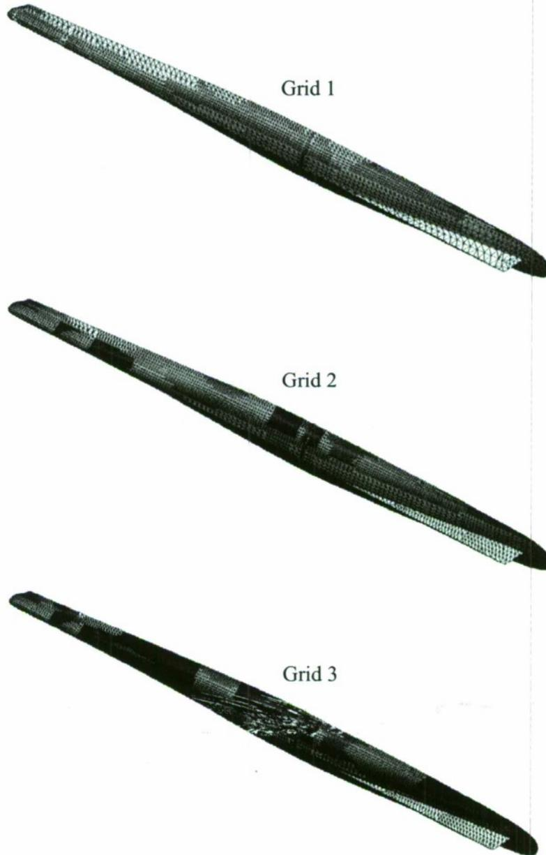
**Figure 4. Hull discretizations used for TSD10 predictions in IHDE for three different mesh densities, corresponding to for JHSS Model 5653 Baseline Bulb at design displacement.**
