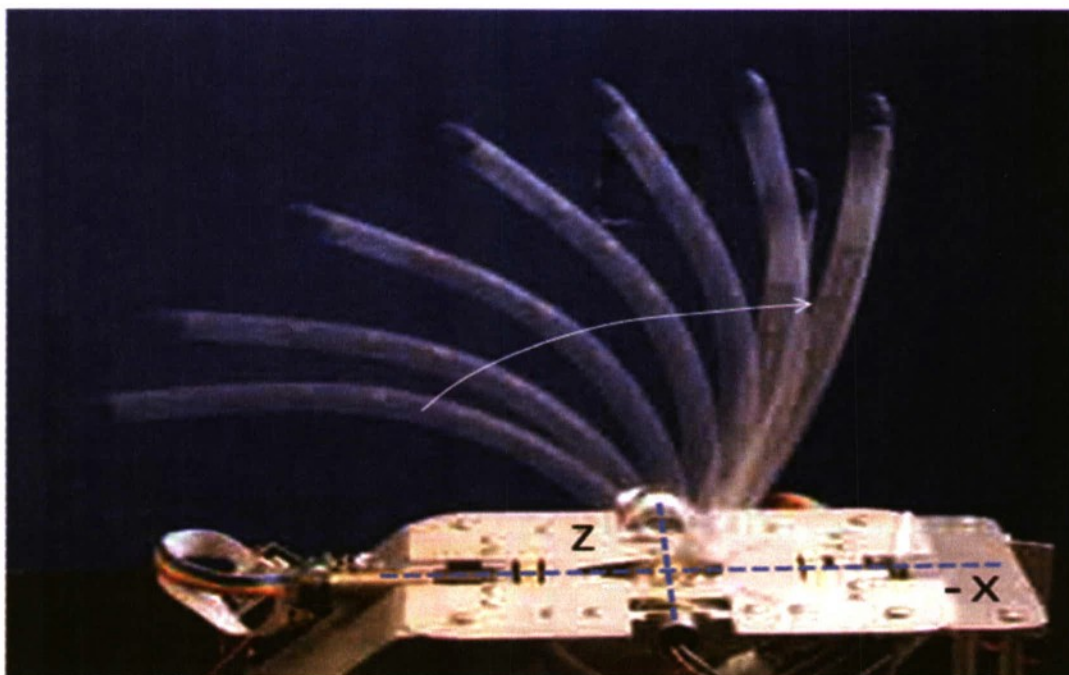
Figure 12. Strobe Picture of the Cilium in the Apparatus Shown in Figure 11 (Return stroke is shown; -X is upstream direction.)
