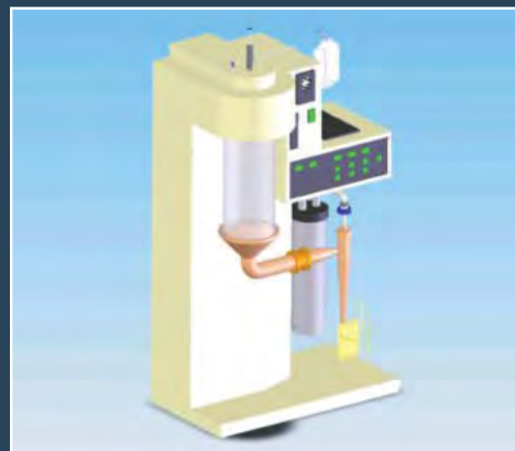
Drawing of a spray-drying device that uses heated nitrogen gas to dry biologicals in <15 msec without damaging labile proteins.
