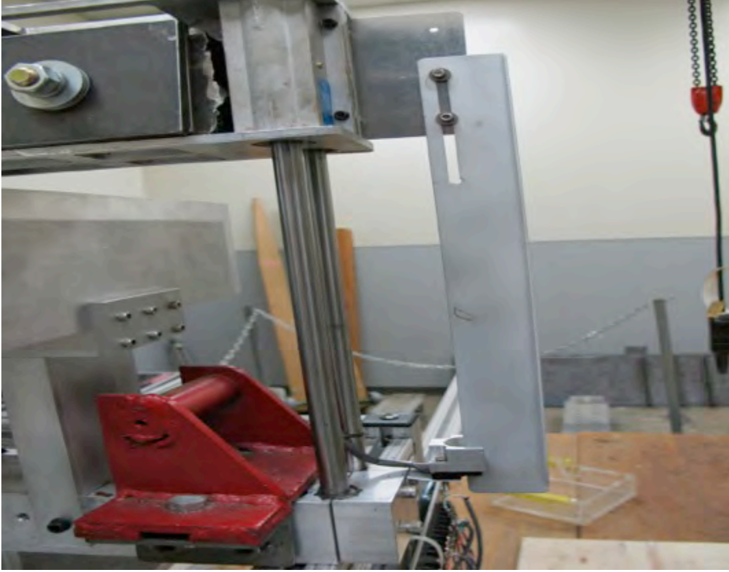
Figure 3. Trigger mechanism and sensor.
