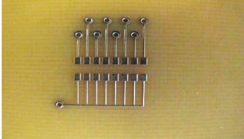
Figure 10. PCB card mounting pad w/o resistor pack.
