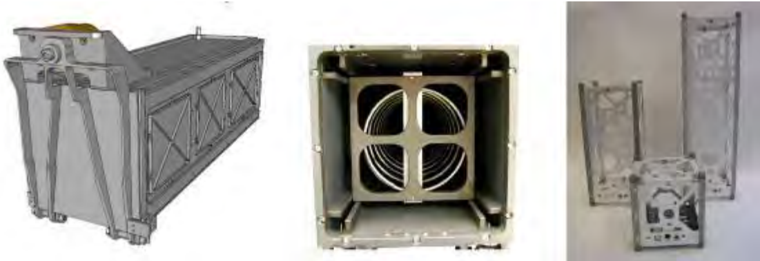
Figure 13. P-POD and CubeSat Structures (2U, 1U, 3U) (From Jenkins, 2010)
