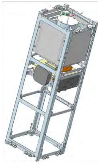
Figure 16. SSA STARE OPTICAL PAYLOAD (NPS CAD model)
