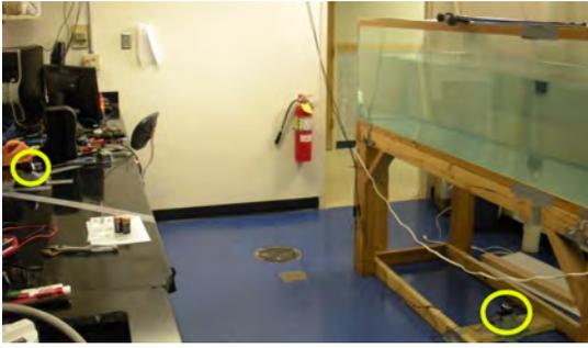
Fig. 1. Camera positions are circled in yellow. One faces the side of the tank, and two view the bottom.
