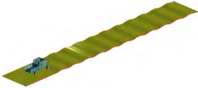
Figure 9. Class 3 truck traversing a 50 m long terrain profile with superimposed periodic bumps.
