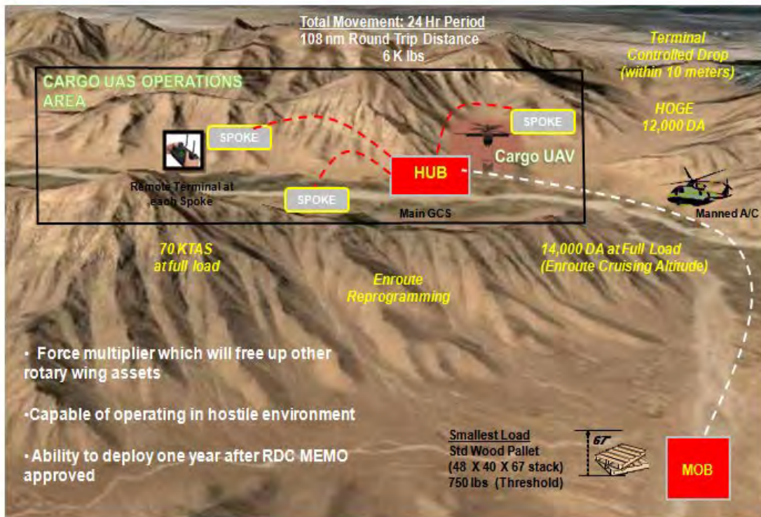
Figure 2. UAS CONOPS (From: E. N. Pratson, personal communication, June 12, 2011)
