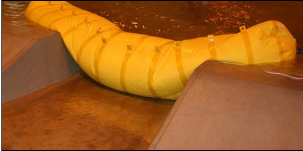
Figure 2.35. Deep-breach closure with large tube filled to 60% fill volume.
