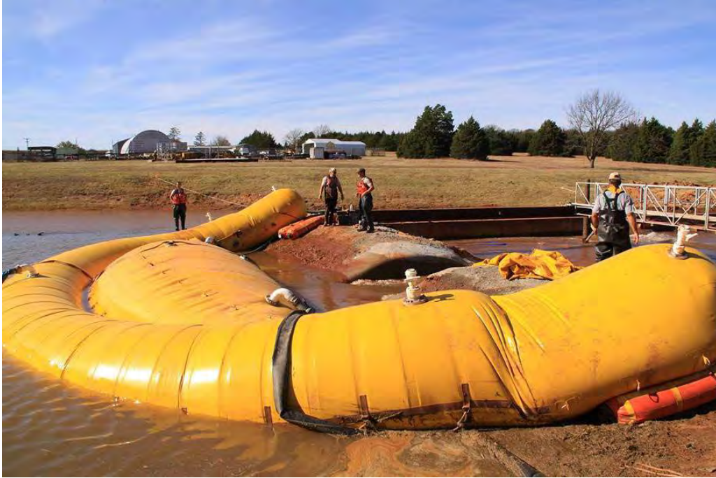
Figure 3.4. Test of the modified ARCH system at Stillwater, Oklahoma, in November 2009. The ballast tank seen behind the apex of the ARCH improved its ability to resist deformation under very high water levels.
