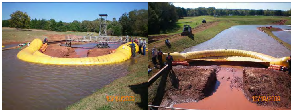
Figure 3.3. Early tests of the ARCH showing its ability to seal the area around a breach to allow the PLUG to be emptied and removed before permanent repairs commence.
