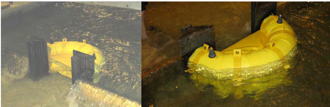
Figure 3.1. Successful laboratory tests of a two-arch system for blocking flow through a simulated “gate” opening. Actual distance spanned by the ARCH in these tests is about 1.5 ft.
