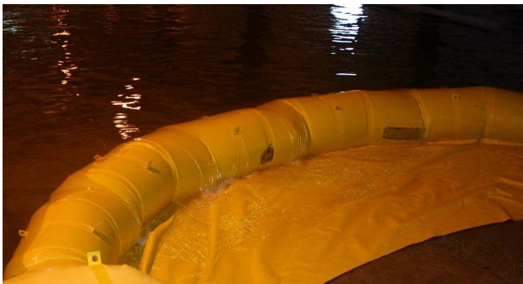
Figure 3.2. Successful small-scale test of a single-arch system for blocking flow across a large open area. The actual distance spanned by the ARCH in this test is about 25 ft.
