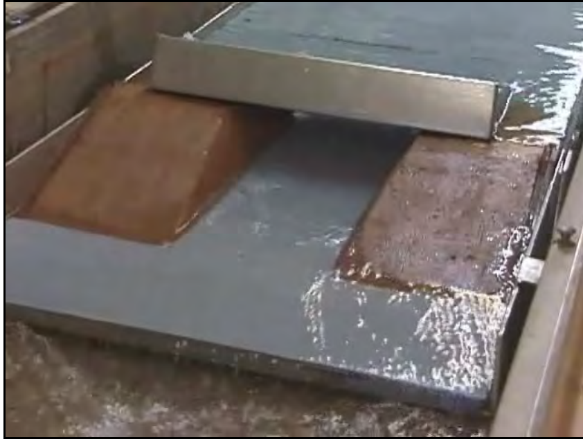
Figure 2.28. Idealized barge floated into position on small-scale levee and ballasted with water.
