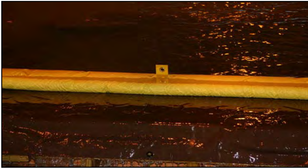
Figure 2.36. Performance of a very long water-filled fabric tube in a wide, shallow breach test in the 1 : 16 scale model.
