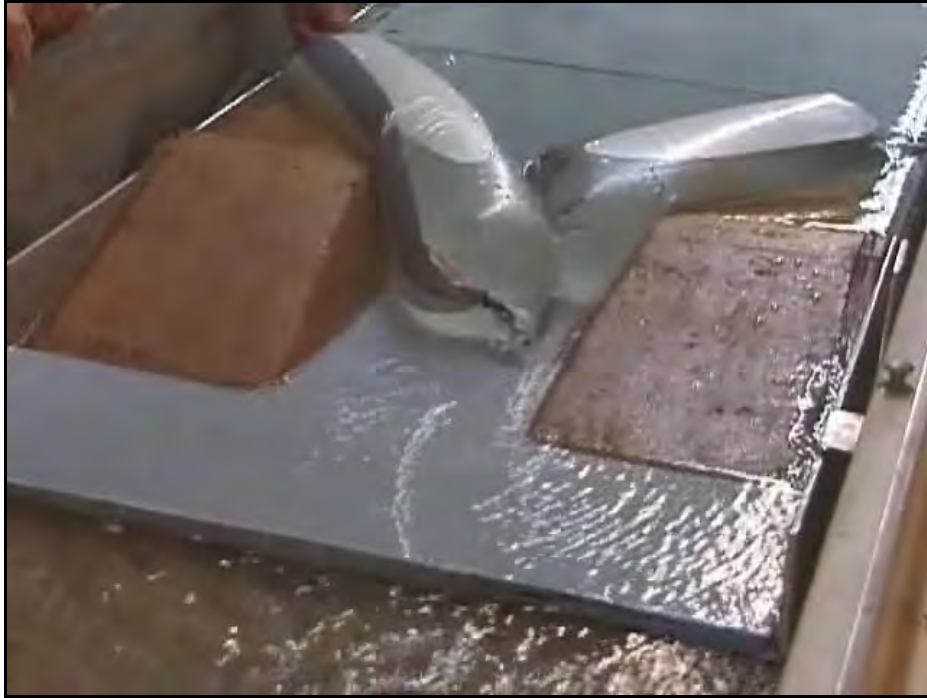
Figure 2.30. Photo of water-filled tube concept using two tubes anchored to either side of a breach in the 1 : 50 scale model basin.
