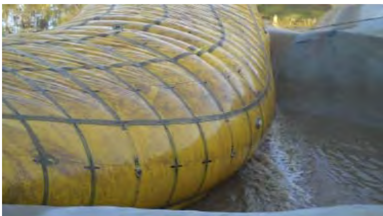
Figure 4.5. Photograph of the same test result as shown in Figure 4.4, except that it is taken from the opposite side of the breach. The curvature of the tube can be clearly seen along with rotational distortion in the longitudinal straps.
