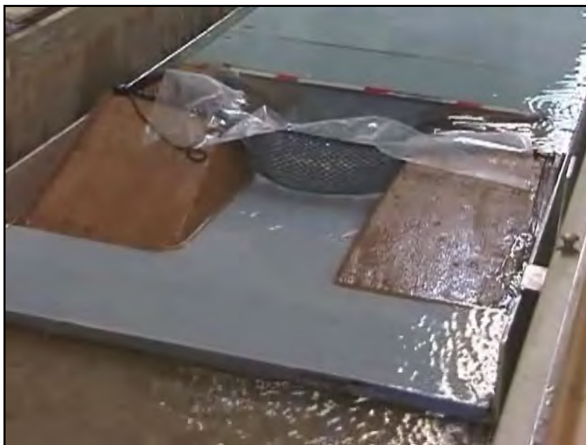
Figure 2.29. Photo of performance of a net anchored on either side of a breach combined with a tarp.
