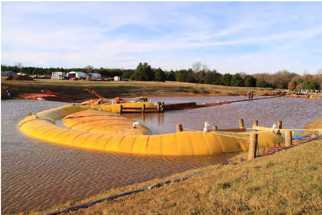
Figure 3.5. Test of the modified ARCH at Stillwater, Oklahoma, in November 2009 showing its ability to block water from flowing into a channel about 40 ft wide with a water depth of about 4 ft.
