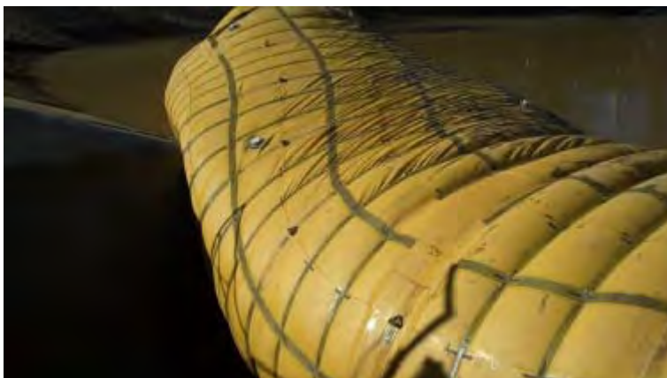
Figure 4.4. Successful test of the PLUG which achieved almost 100% stoppage of flow. The view in this figure is from the downstream side of the breach, with the water that is being held back from the breach shown in the upper right.
