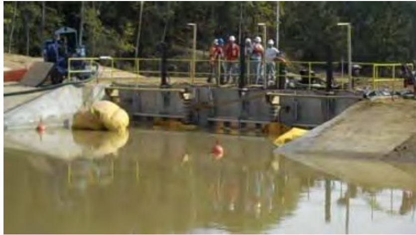
Figure 4.3. First PLUG test culminated in a failure, with substantial damage to the gate protection system and tears to the PLUG.
