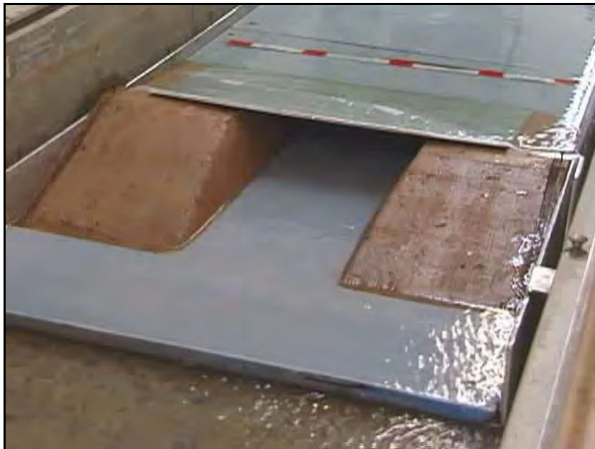
Figure 2.27. Test of a gated structure combined with a tarp showing almost no residual flow.
