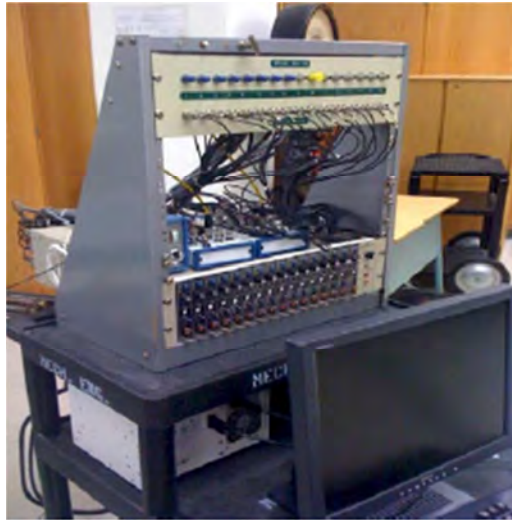
Figure 40. Data Acquisition System
