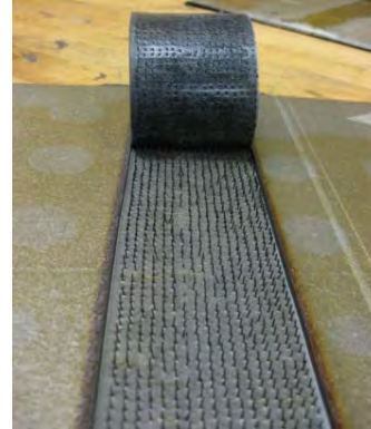
Figure 2.7 Z-Pin Field After the Removal of Rubber Sheet
