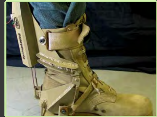
Combat boot add-on biomechanical energy harvesting device, SPaRK
