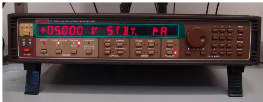
Figure 34 Keithley 237 high-voltage source-measure unit
