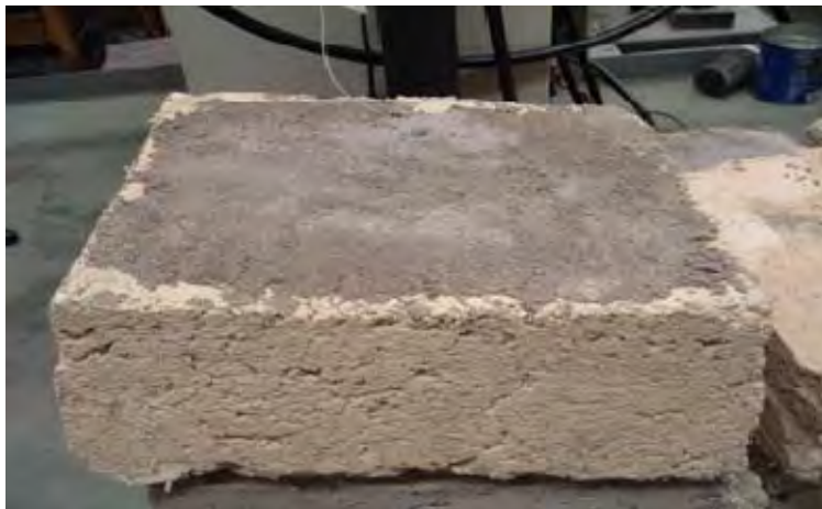
Figure 7: Papercrete Block with Mortar (From The Center for Alternative Building Studies, 2005)
