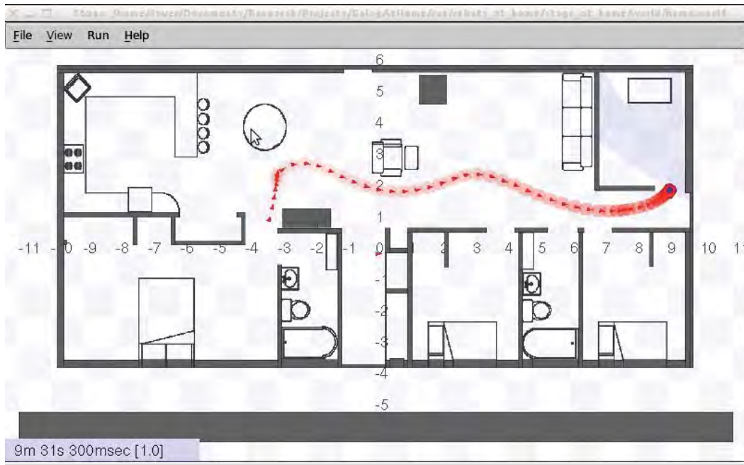
Figure 1. Sending the robot from the “master bedroom” to the “study” requires passing through the “dining room”, “living room”, and a number of doorways.
