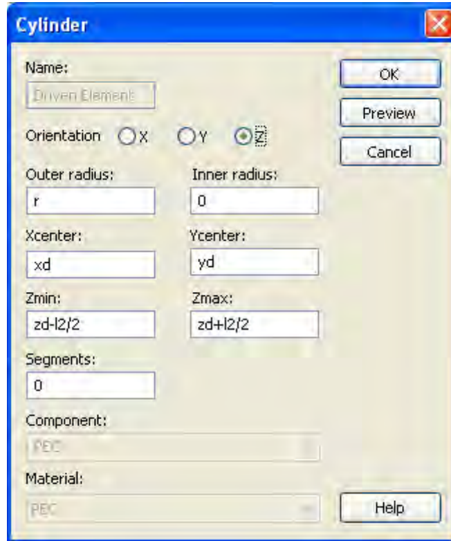
Figure 18. Properties of Cylinder object used to construct dipole antenna.
