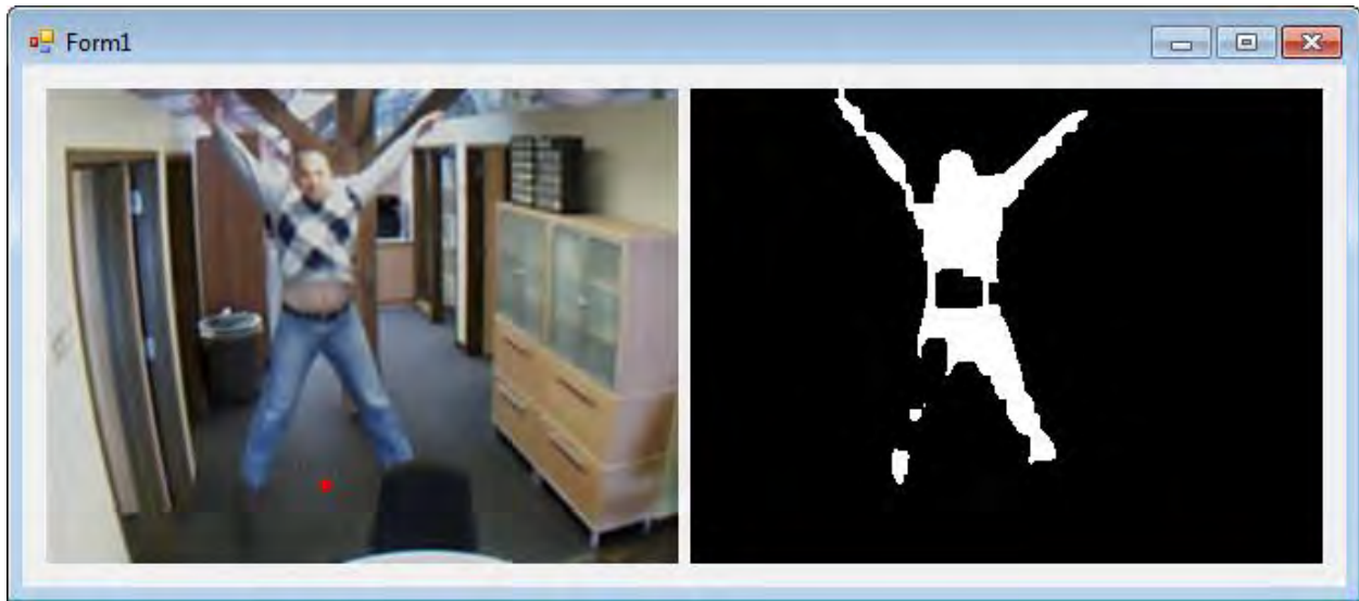
Figure 32: Primordial In-House Tracking System in Use
