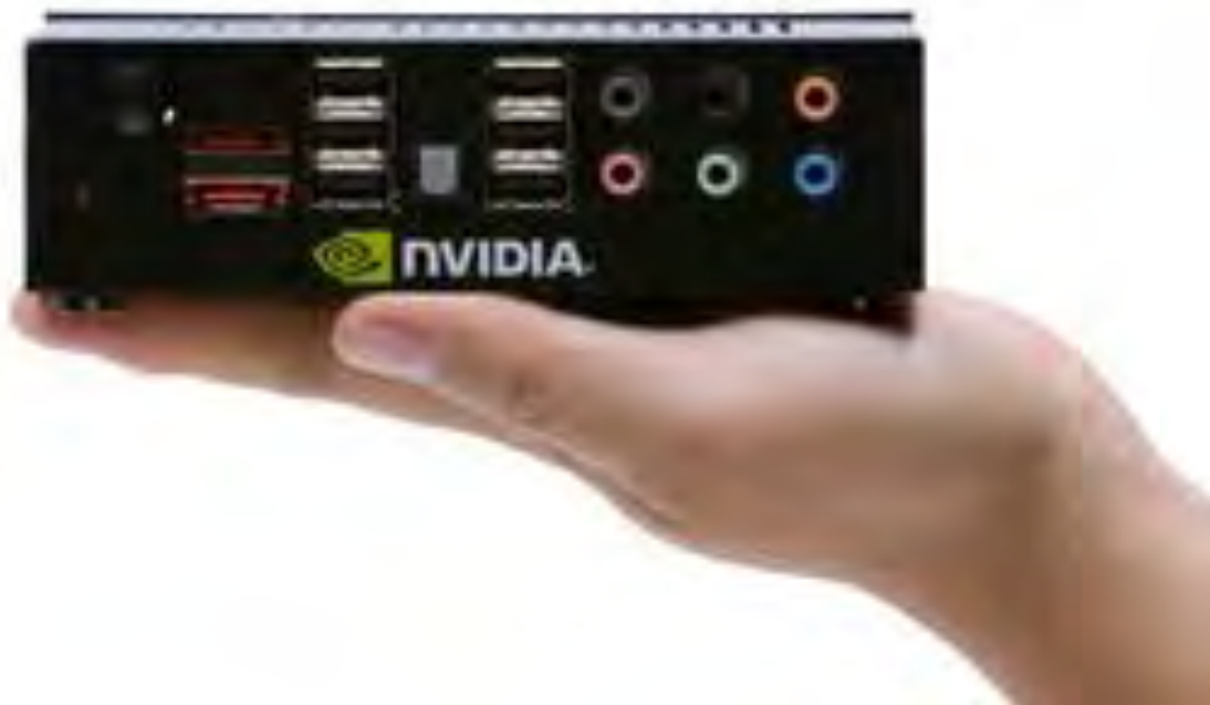
Figure 10: Example of a Mini-PC That Employs the Nvidia Ion Architecture
