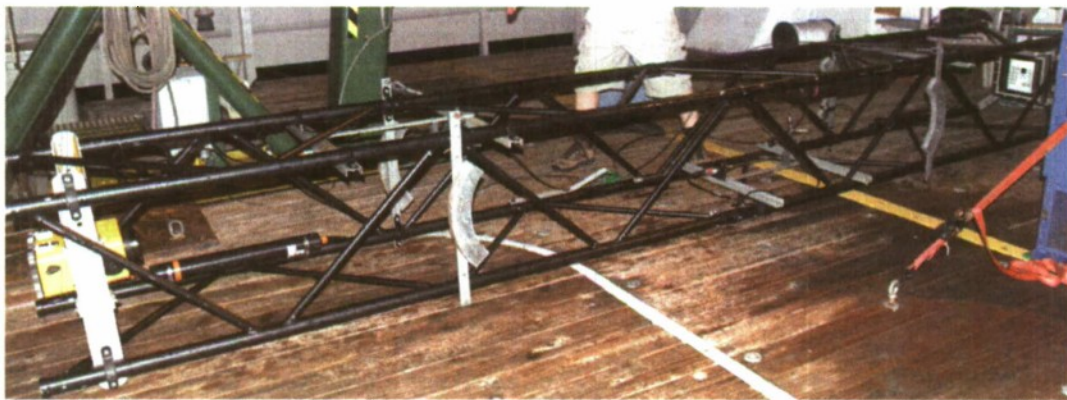
Figure 2. IMAST night deployment configuration: imaging camera and housing (left end of the frame); active target made out of iPad (right end of the frame); details on other sensors including Vector refer to text.
