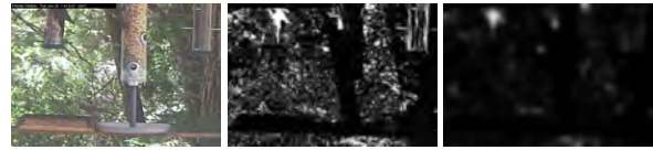
Figure 12. Using the implicit warp model, the increasing patch width w reduces false positives, by enforcing a spatial warping across larger areas of the image.
